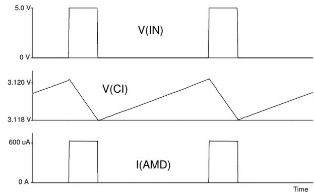
Figure 4: Steady-state APC,  $f(IN) = 100$  kHz (1:4),
