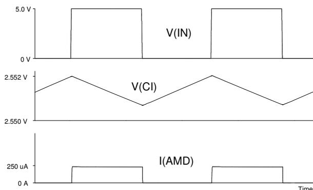
Figure 3: Steady-state APC,  $f(IN) = 100$  kHz (1:1),
