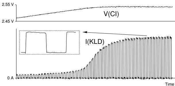
Figure 6: Turn-on behaviour, detailed view  $f(IN) = 100$  kHz (1:1), CI = 470 nF, RSET = 10 kΩ
