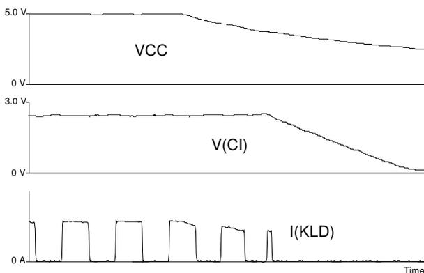
Figure 7: Turn-off behaviour,  $f(IN) = 100$  kHz (1:1), CI = 470 nF, RSET = 10 kΩ
