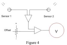
In practice, the output of the amplifier is read by an Analog to Digital Converter (ADC) and the offsets are applied digitally. Two variants of this concept have been flown, one with fixed wingtip sensors and the second with a movable sensor plate.
