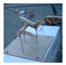
Figure 8. Movable Roll plate sensor.
