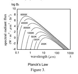
Wavelengths of 7.5 to 13.5 microns correspond roughly to the blackbody radiation from objects in the +75 to -75 degrees Centigrade range. A silicon filter prevents these thermopiles from responding to short wavelengths from the sun (6000 degrees Kelvin – around 550 nM peak).
