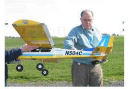
Figure 12. Controls ground test. Note the aileron & elevator deflection while the vehicle is stationary.
