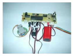
Figure 14. Digital section with ASI and Altitude sensors, servo, RS-232 interface and battery pack.
