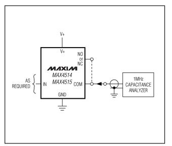
Figure 4. NO, NC, and COM Capacitance
