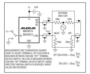
Figure 3. Off-Isolation and On-Loss
