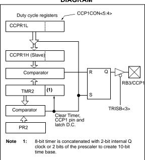
A PWM output (Figure 9-4) has a time base (period) and a time that the output stays high (duty cycle). The frequency of the PWM is the inverse of the period (frequency = 1/period).
