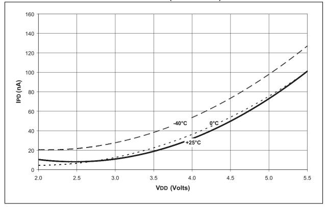
FIGURE 18-2: TYPICAL BASELINE IPD vs. VDD (85°C)
