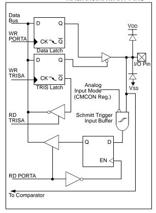
FIGURE 5-2: BLOCK DIAGRAM OF RA2/AN2/VREF PIN
