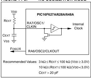
The RC Oscillator mode has two options that control the unused OSC2 pin. The first allows it to be used as a general purpose I/O port. The other configures the pin as an output providing the Fosc signal (internal clock divided by 4) for test or external synchronization purposes.
