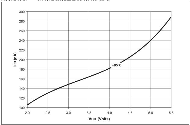
FIGURE 18-3: TYPICAL BASELINE CURRENT IPD vs. VDD (125°C)
