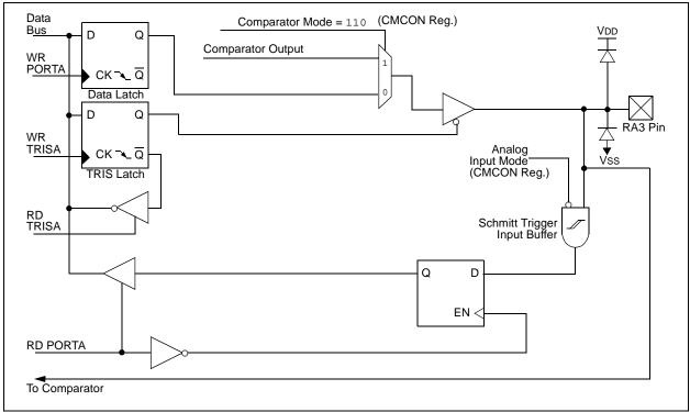
FIGURE 5-4: BLOCK DIAGRAM OF RA4/T0CKI/CMP2 PIN
