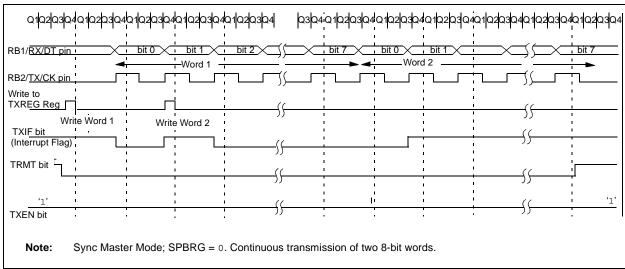
FIGURE 12-9: SYNCHRONOUS TRANSMISSION (THROUGH TXEN)
