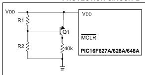
Note 1: This brown-out circuit is less expensive, albeit less accurate. Transistor Q1 turns off when VDD is below a certain level such that:
