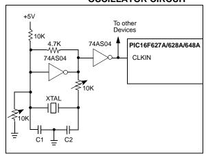
Figure 14-3 shows a series resonant oscillator circuit. This circuit is also designed to use the fundamental frequency of the crystal. The inverter performs a 180° phase shift in a series resonant oscillator circuit. The 330  $k\Omega$  resistors provide the negative feedback to bias the inverters in their linear region.
