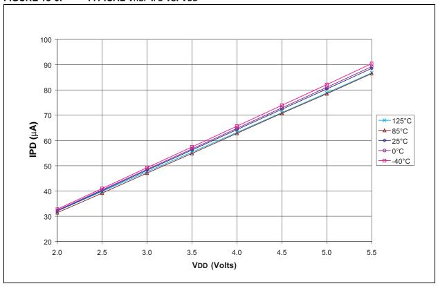
FIGURE 18-7: TYPICAL WDT IPD vs. VDD
