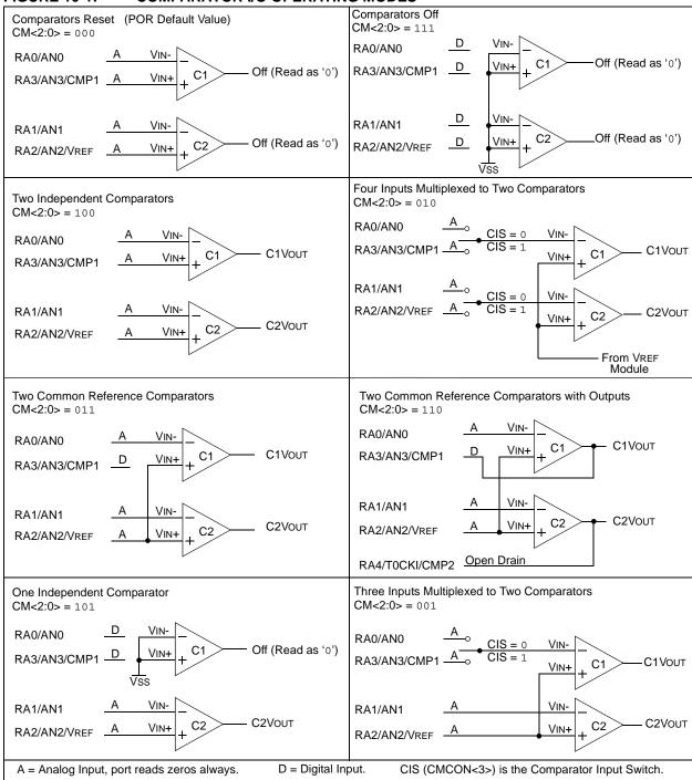
The code example in Example 10-1 depicts the steps required to configure the Comparator module. RA3 and RA4 are configured as digital output. RA0 and RA1 are configured as the V- inputs and RA2 as the V+ input to both comparators.
