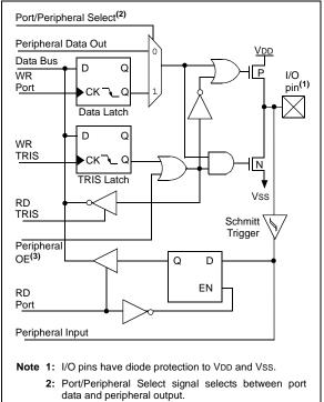
3: Peripheral OE (Output Enable) is only activated if Peripheral Select is active.
