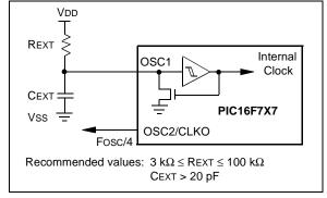
The RCIO Oscillator mode (Figure 4-5) functions like the RC mode, except that the OSC2 pin becomes an additional general purpose I/O pin. The I/O pin becomes bit 6 of PORTA (RA6).
