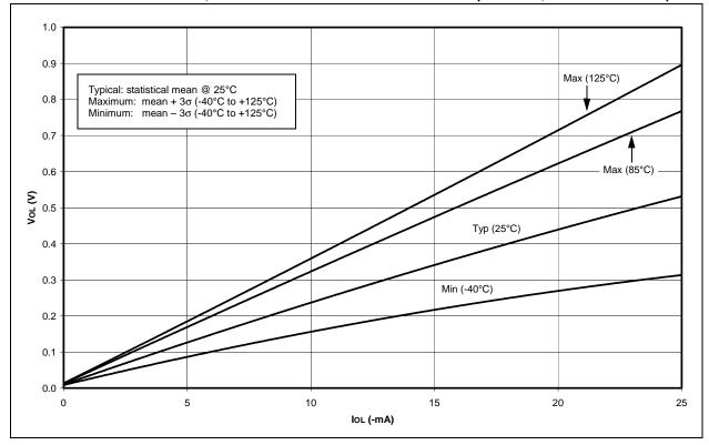
FIGURE 19-21: TYPICAL, MINIMUM AND MAXIMUM Vol vs. lol (VDD = 5V, -40°C TO +125°C)
