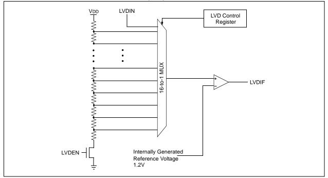
The LVD module has an additional feature that allows the user to supply the sense voltage to the module from an external source. This mode is enabled when bits LVDL3:LVDL0 are set to '1111'. In this state, the comparator input is multiplexed from the external input pin, LVDIN (Figure 15-5). This gives users flexibility because it allows them to configure the Low-Voltage Detect interrupt to occur at any voltage in the valid operating range.
