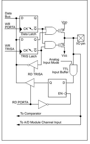
FIGURE 5-2: BLOCK DIAGRAM OF RA3/AN3/VREF+ PIN
