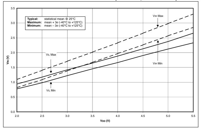
FIGURE 19-25: MINIMUM AND MAXIMUM VIN vs. VDD (I<sup>2</sup>C<sup>™</sup> INPUT, -40°C TO +125°C)
