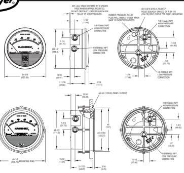
\*The blowout plug is not used on models above 180 inches of water pressure, medium or high pressure models, or on gages which require an elastomer other than silicone for the diaphragm.
