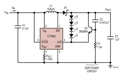
Figure 7. Soft-Start Circuit for the LT1932
