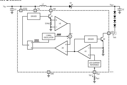
Figure 1. LT1932 Block Diagram
