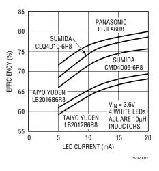
Figure 2. Efficiency for Several Different Inductor Types
