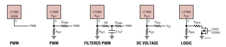
Figure 6. Five Methods of LED Dimming
