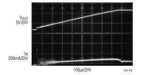
Figure 9. Input Current at Start-Up with Soft-Start
