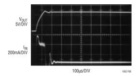
Figure 8. Input Current at Start-Up Without Soft-Start
