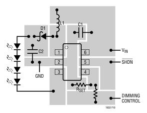
Figure 10. Recommended Component Placement
