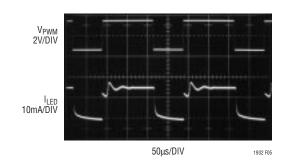
Figure 5. PWM Dimming Using the SHDN Pin
