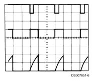
$$\begin{split} &V_{CC}=5V\\ &\text{TIME}=0.1\text{ ms/DIV}.\\ &R_A=9.1\text{k}\Omega\\ &C=0.01\mu\text{F} \end{split}$$
