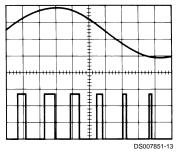
$V_{CC} = 5V$ Top Trace: Modulation 1V/Div. TIME = 0.2 ms/DIV. Bottom Trace: Output Voltage 2V/Div.  $R_A = 9.1k\Omega$  $C = 0.01 \mu F$
