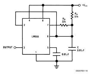
FIGURE 14. 50% Duty Cycle Oscillator
