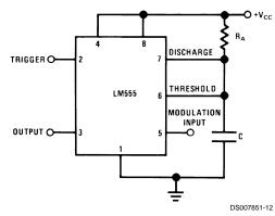
FIGURE 8. Pulse Width Modulator
