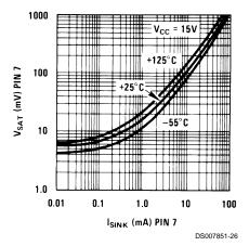
Discharge Transistor (Pin 7) Voltage vs. Sink Current
