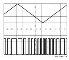
$V_{CC} = 5V$ TIME = 0.1 ms/DIV. Top Trace: Modulation Input 1V/Div. Bottom Trace: Output 2V/Div.
