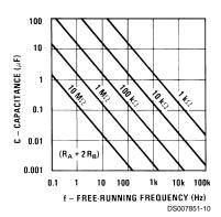
FIGURE 6. Free Running Frequency
