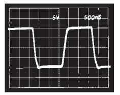
Figure 4. The Pulse Response of the 3-Op Amp Instrumentation Amplifier. Gain = 1, Horizontal Scale = 0.5 ms/Div and Vertical Scale = 5 V/Div.
