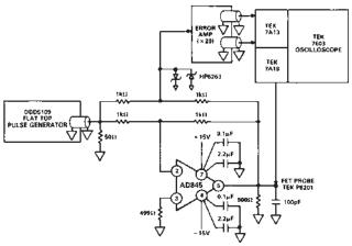
Figure 2. Settling Time Test Circuit
