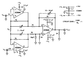
Figure 3. High Performance, High Speed Instrumentation Amplifier
