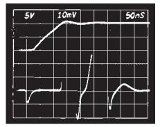
Figure 1. Settling Characteristics 0 V to 10 V Step Upper Trace: Output of AD845 Under Test (5 V/Div) Lower Trace: Error Voltage (1 mV/Div)
