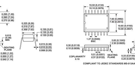
COMPLIANT TO JEDEC STANDARDS MO-095AA CONTROLLING DIMENSIONS ARE IN INCHES; MILLIMETER DIMENSIONS (IN PARENTHESES) ARE ROUNDED-OFF INCH EQUIVALENTS FOR REFERENCE ONLY AND ARE NOT APPROPRIATE FOR USE IN DESIGN
