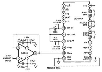
Figure 7. AD845 As ADC Unity Gain Buffer
