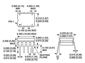
CONTROLLING DIMENSIONS ARE IN INCHES; MILLIMETERS DIMENSIONS (IN PARENTHESES) ARE ROUNDED-OFF INCH EQUIVALENTS FOR REFERENCE ONLY AND ARE NOT APPROPRIATE FOR USE IN DESIGN
