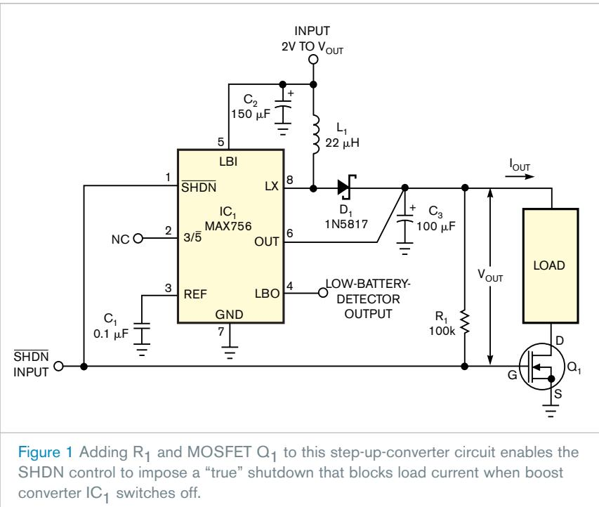
**Figure 1** Adding R<sub>1</sub> and MOSFET Q<sub>1</sub> to this step-up-converter circuit enables the SHDN control to impose a “true” shutdown that blocks load current when boost converter IC<sub>1</sub> switches off.
