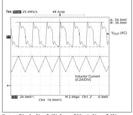
Output Ripple,  $V_{IN}$ =2.6V,  $I_{LOAD}$ =200mA,  $V_{OUT}$ =5.0V
