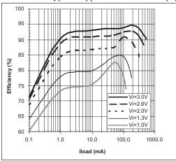
Efficiency vs. Load Current,  $V_{OUT}$ =3.3V
