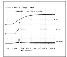
Startup,  $V_{IN}$ =4.2V,  $V_{OUT}$ =5.0V,  $R_{LOAD}$  = 100 $\Omega$
