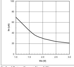
No Load Battery Current, Vout=3.3V
