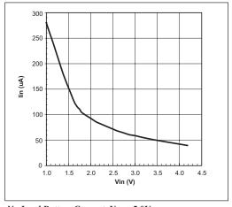
No Load Battery Current, V<sub>OUT</sub>=5.0V
