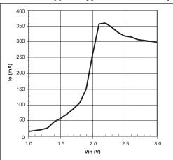
Maximum Resistive Load Current in Startup,  $V_{OUT}$ =3.3V
