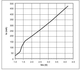
Maximum Resistive Load Current in Startup,  $V_{OUT}$ =5.0V
