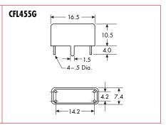
Note: For safety purposes, connect the output of filters to the IF amplifier through a DC blocking capacitor. Avoid applying a direct current to the output of ceramic filters.
