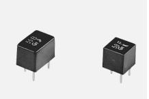
The CFUS Y lines of ceramic filters are 4-element devices connected in ladder form while the CFWS Y455 filters contain 6-elements. These highly selective filters are designed to address the G.D.T. characteristics required in digital communications. The excellent G.D.T. characteristics allow these filters to be utilized in areas such as the mobile cellular markets as well as a variety of stereo applications. Available in 450kHz and 455kHz versions.
