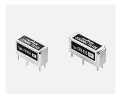
The following lines of filters are high performance devices that achieve ultimate stopband attenuation through the use of multiple piezoelectric elements connected in ladder form. A few of the recommended applications for these filters include high class receivers, SSB communications equipment, pocket pagers and mobile radios.
