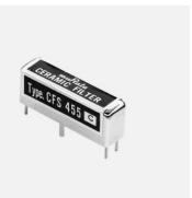
The following lines of filters are high performance devices that achieve ultimate stopband attenuation through the use of multiple piezoelectric elements connected in ladder form. A few of the recommended applications for these filters include high class receivers, SSB communications equipment, pocket pagers and mobile radios.
