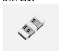
The CFECV Series are small, high performance and super thin (1.5mm) filters. Piezoelectric element is connected in the sandwich shape by heat resistant substrate. The filters exhibit flat G.D.T characteristic in pass band. The filters are recommended for digital communication application and are perfect in hand held cellular phones, pocket cordless phones, etc.
