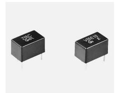
The CFVM line of ceramic filters are 7-element devices connected in ladder form while the CFZM line of filters contain 9-elements. These highly selective filters offer improved stopband attenuation and are recommended for use in a variety of applications. Available in 450kHz and 455kHz versions.
