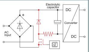
Simplified schematic of the Dimension Q-Series Inrush current limitation with pulsed charging of the input capacitor.
