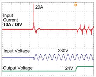
"Cold start" of a 24V, 10A power supply with NTC resistor inrush current limiting typ. peak inrush current = 29A
