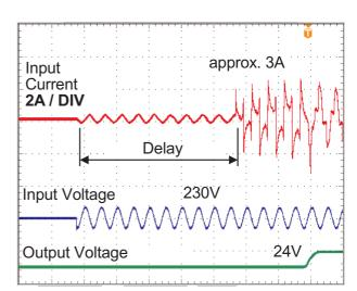
24V, 10A power supply from the PULS Dimension series with pulsed charging of the input capacitor typ. peak inrush current = 3A
