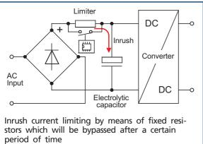
summate and load the MCBs and the system voltage heavily. The delay in the PULS Dimension Q series anticipates this initial current surge and switches on a few 100 ms later. This gives
