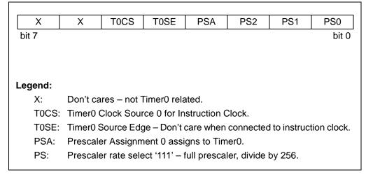
Lesson 9 configures Timer0 with the Prescaler for a maximum delay on Timer0. The prescaler will divide the processor clock by 256 and Timer0 will divide that by 256 again. Thus, Timer0 Flag will be set every 65536  $\mu s$  (0.0000001 second \* 256 \* 256), or about 15 times a second. The main program sits in a loop waiting for the rollover and when it does, it increments the display and then loops back.
