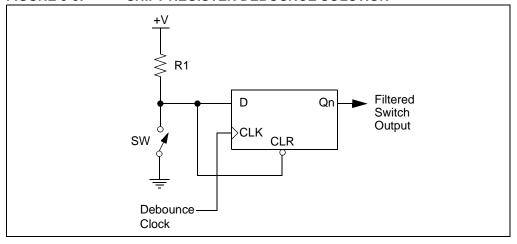
One of the simplest ways to switch debounce is to sample the switch until the signal is stable or continue to sample the signal until no more bounces are detected. How long to continue sampling requires some investigation. However, 5 mS is usually plenty long, while still reacting fast enough that the user won't notice it.
