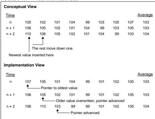
Calculating averages in a mid-range PICmicro is best accomplished by using the FSR to keep track of where the next value will be inserted. This ensures the oldest value is always overwritten with the newest and doesn't waste time moving values within the memory.
