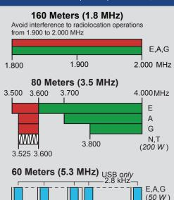
5330.5 5346.5 5366.5 5371.5 5403.5 kHz General, Advanced, and Amateur Extra licensees may use the following five channels on a secondary basis with a maximum effective radiated power of 50 W PEP relative to a half wave dipole. Only upper sideband suppressed carrier voice transmissions may be used. The frequencies are 5330.5, 5346.5, 5366.5, 5371.5 and 5403.5 kHz. The occupied bandwidth is limited to 2.8 kHz centered on 5332, 5348, 5368, 5373, and 5405 kHz respectively.
