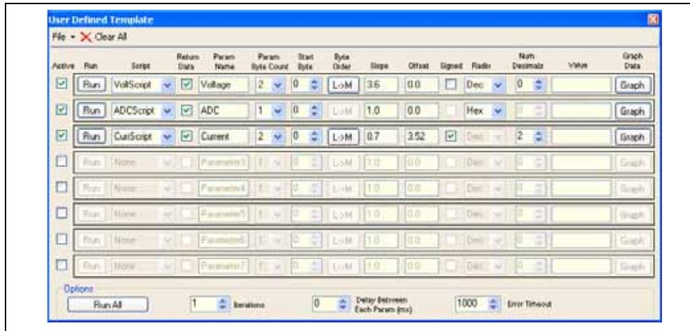
Create the Parameter Template by filling in each line. Each line is a single parameter, a value read converted to value displayed. The *inputs* below define how a particular parameter is interpreted.
