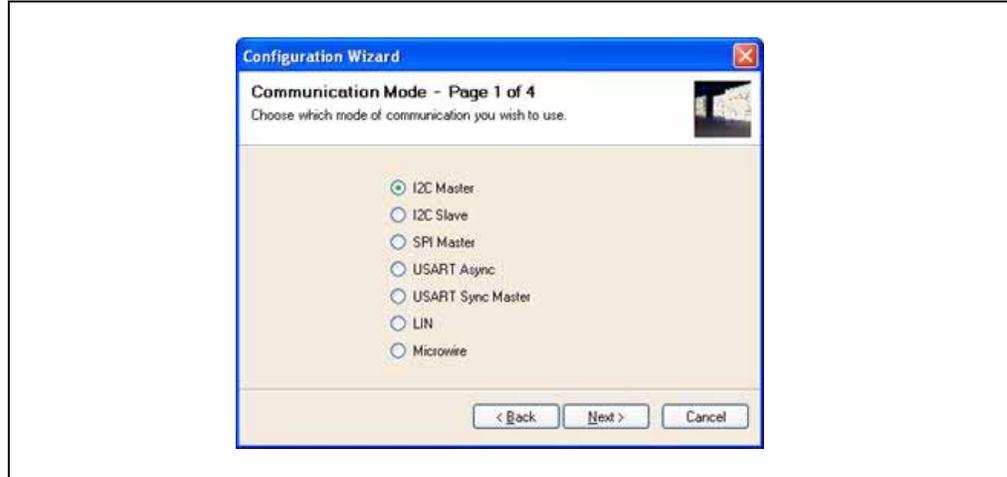
In this example, I<sup>2</sup>C Master Communication mode is selected. The Configuration Wizard Page 2 of 4, as shown in Figure 3-4, allows you to select the bus speed. A more comprehensive list of bus speeds can be chosen from the Configuration window by selecting *PICKit Serial Analyzer > Configure Communications Mode* from the menu bar.
