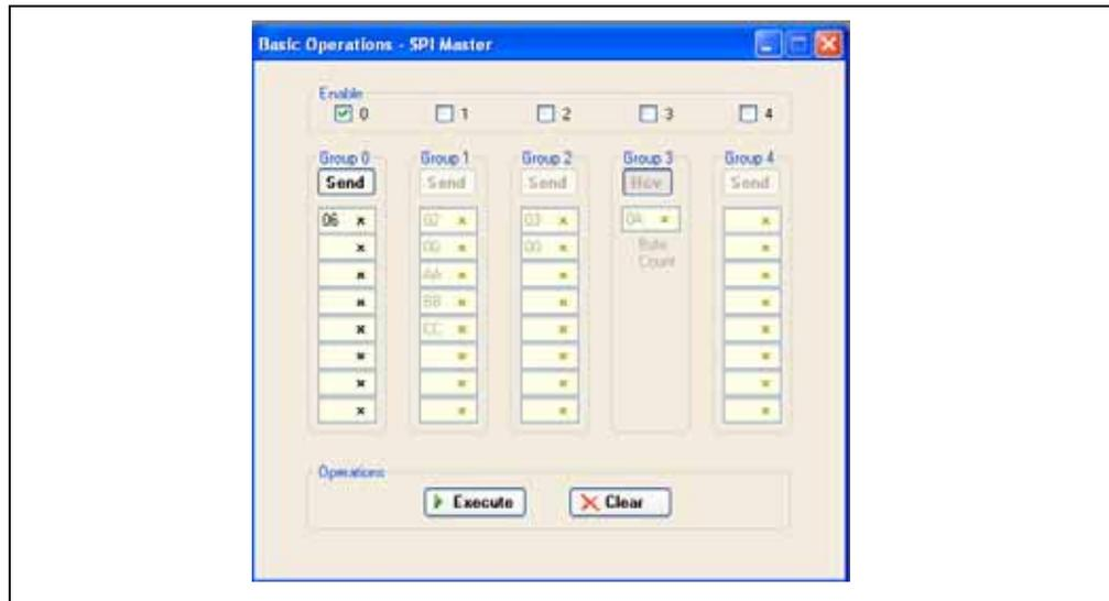
Once the WREN latch has been enabled, data can be written to the 25LC020A. Figure 7-6 shows that Group 0 has been disabled, and Group 1 enabled. Clicking on the **Execute** button will send the Write command (0x02), the memory address (0x00), followed by three bytes of data: 0xAA, 0xBB and 0xCC. The command will be logged in the Transactions window.
