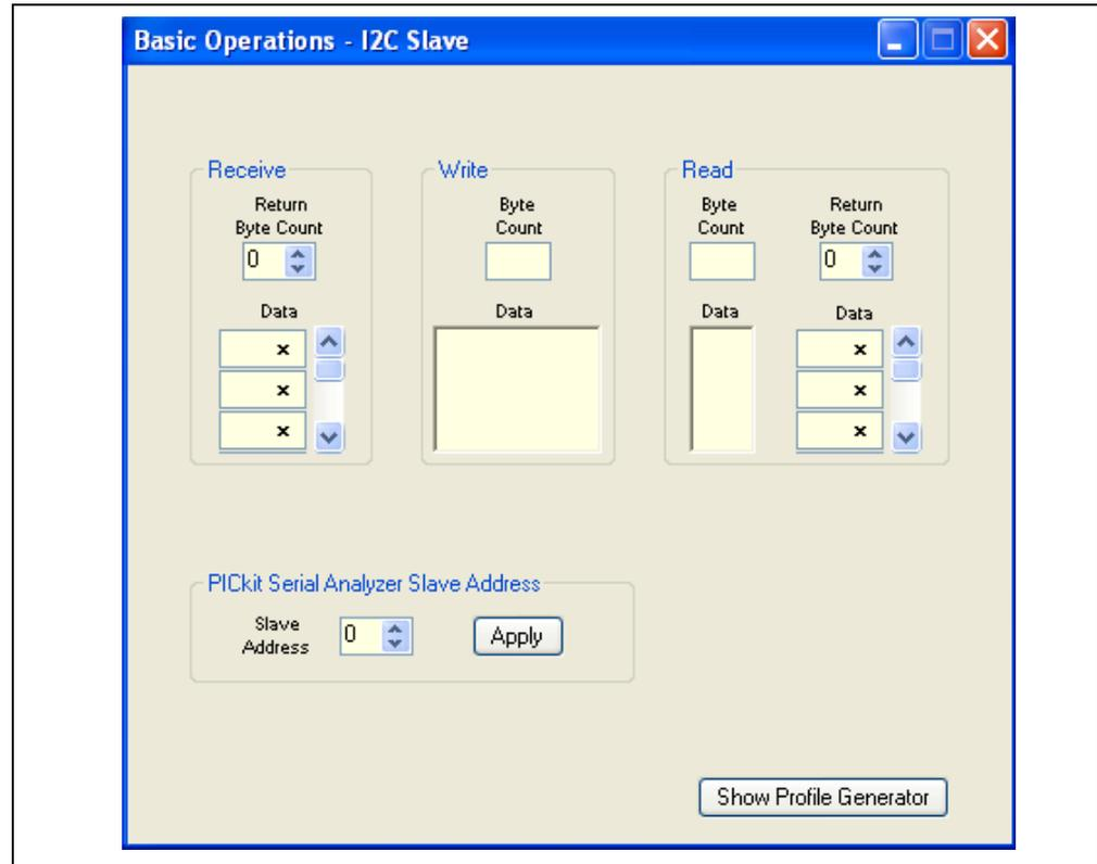
**Receive** responds to a basic Receive request from the master. In Return Byte Count, enter the number of bytes a Receive request will respond with, then enter the data to be returned in the data array. The Basic page limits you to eight bytes of returned data.
