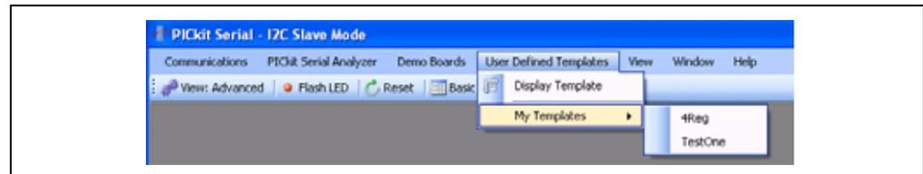
This implementation of the User Defined Template differs from the one in the prior release of PICKit Serial Analyzer in that you create and run the template on the same form. This allows for a great deal of run time flexibility. For example, you can change any of the *inputs* from **Section 10.3 “Creating and Using Templates”** while you are running the scripts in a loop.
