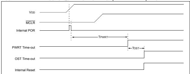
FIGURE 14-5: TIME-OUT SEQUENCE ON POWER-UP (DELAYED MCLR): CASE 2
