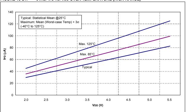
FIGURE 18-22: CVREF IPD vs. VDD OVER TEMPERATURE (LOW RANGE)
