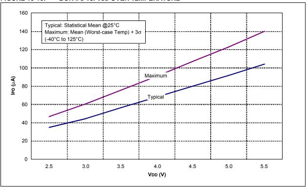
FIGURE 18-17: TYPICAL WDT IPD vs. VDD OVER TEMPERATURE
