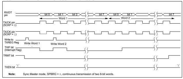
FIGURE 12-11: SYNCHRONOUS TRANSMISSION (THROUGH TXEN)
