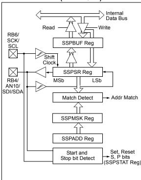
The SSP module has six registers for the I<sup>2</sup>C operation, which are listed below.
