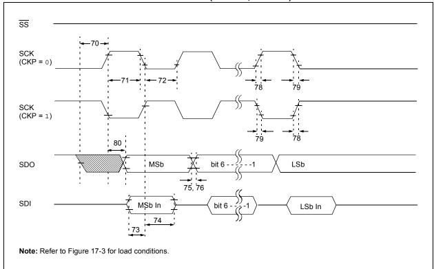
FIGURE 17-13: SPI MASTER MODE TIMING (CKE = 1, SMP = 1)
