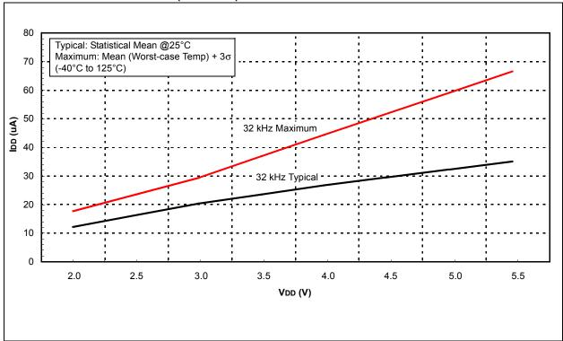
FIGURE 18-8: TYPICAL IDD vs. VDD OVER FOSC (EXTRC MODE)
