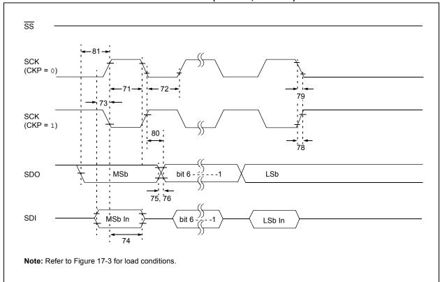
FIGURE 17-14: SPI SLAVE MODE TIMING (CKE = 0)
