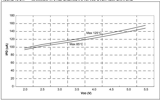
FIGURE 18-25: T1OSC IPD vs. VDD OVER TEMPERATURE (32 kHz)
