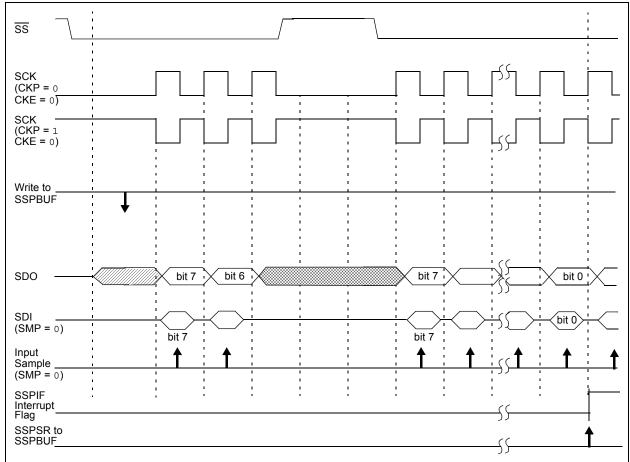
FIGURE 13-5: SPI MODE WAVEFORM (SLAVE MODE WITH CKE = 0)
