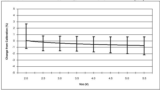
FIGURE 18-41: TYPICAL HFINTOSC FREQUENCY CHANGE vs. VDD (125°C)
