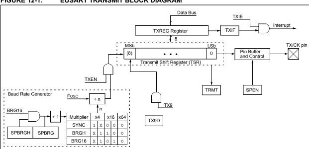
FIGURE 12-1: EUSART TRANSMIT BLOCK DIAGRAM
