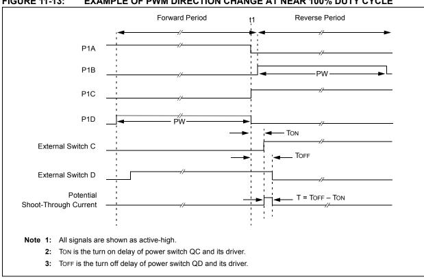
FIGURE 11-13: **EXAMPLE OF PWM DIRECTION CHANGE AT NEAR 100% DUTY CYCLE**
