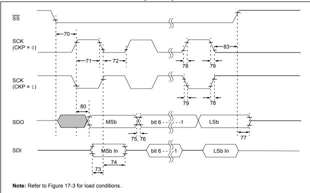
FIGURE 17-15: SPI SLAVE MODE TIMING (CKE = 1)
