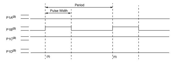
Note 1: At this time, the TMR2 register is equal to the PR2 register.
