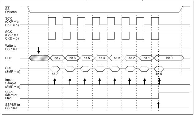
FIGURE 13-6: SPI MODE WAVEFORM (SLAVE MODE WITH CKE = 1)
