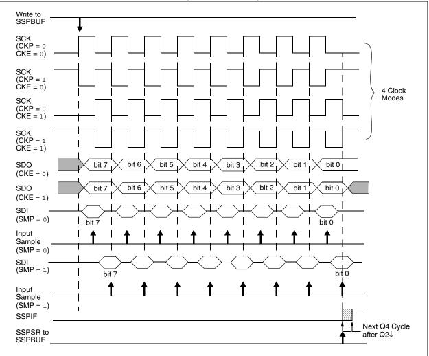
FIGURE 17-3: SPI MODE WAVEFORM (MASTER MODE)
