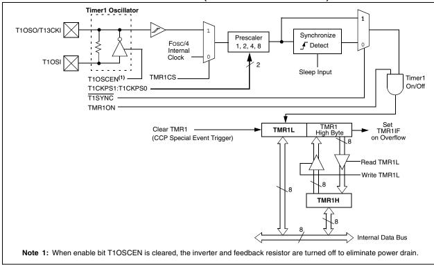
cycle (Fosc/4). When the bit is set, Timer1 increments on every rising edge of the Timer1 external clock input or the Timer1 oscillator, if enabled.
