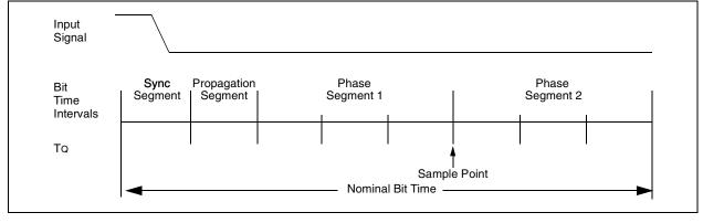
The Nominal Bit Time can be thought of as being divided into separate, non-overlapping time segments. These segments (Figure 23-4) include:
