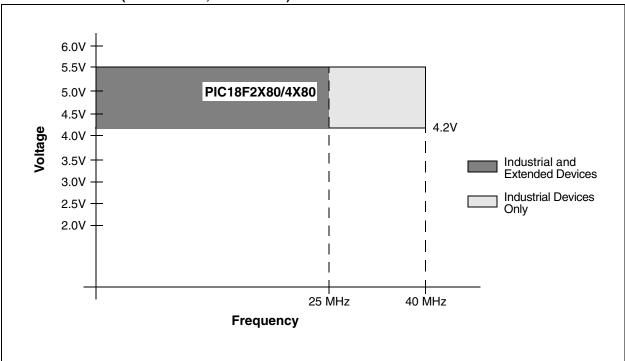
FIGURE 27-2: PIC18LF2480/2580/4480/4580 VOLTAGE-FREQUENCY GRAPH (INDUSTRIAL)
