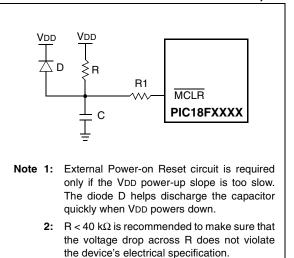
R1 ≥ 1 kΩ will limit any current flowing into MCLR from external capacitor C, in the event of MCLR/VPP pin breakdown, due to Electrostatic Discharge (ESD) or Electrical Overstress (EOS).
