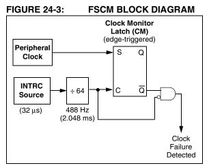
Clock failure is tested for on the falling edge of the sample clock. If a sample clock falling edge occurs while CM is still set, a clock failure has been detected (Figure 24-4). This causes the following:
