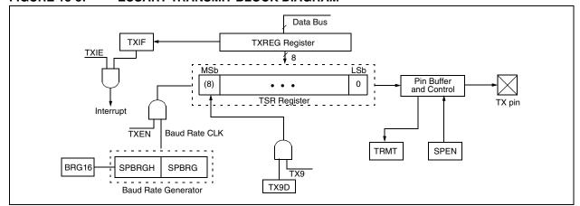
FIGURE 18-4: ASYNCHRONOUS TRANSMISSION
