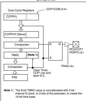
A PWM output (Figure 15-4) has a time base (period) and a time that the output stays high (duty cycle). The frequency of the PWM is the inverse of the period (1/period).
