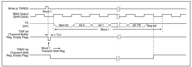
FIGURE 18-5: ASYNCHRONOUS TRANSMISSION (BACK-TO-BACK)
