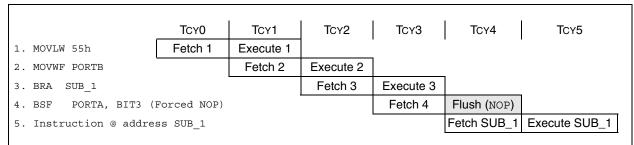
**Note:** All instructions are single cycle, except for any program branches. These take two cycles since the fetch instruction is "flushed" from the pipeline while the new instruction is being fetched and then
