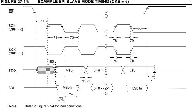
FIGURE 27-14: **EXAMPLE SPI SLAVE MODE TIMING (CKE = 0)**
