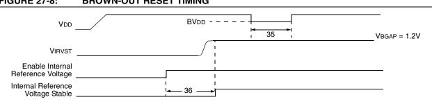
TABLE 27-10: RESET, WATCHDOG TIMER, OSCILLATOR START-UP TIMER, POWER-UP TIMER AND BROWN-OUT RESET REQUIREMENTS
