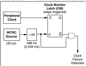
Clock failure is tested for on the falling edge of the sample clock. If a sample clock falling edge occurs while CM is still set, a clock failure has been detected (Figure 24-4). This causes the following:
