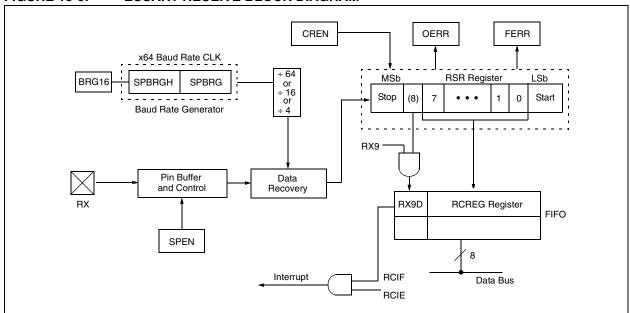
FIGURE 18-7: ASYNCHRONOUS RECEPTION
