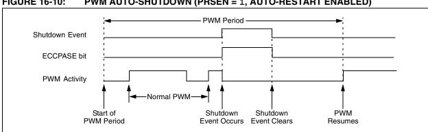
**FIGURE 16-10:** PWM AUTO-SHUTDOWN (PRSEN = 1, AUTO-RESTART ENABLED)
