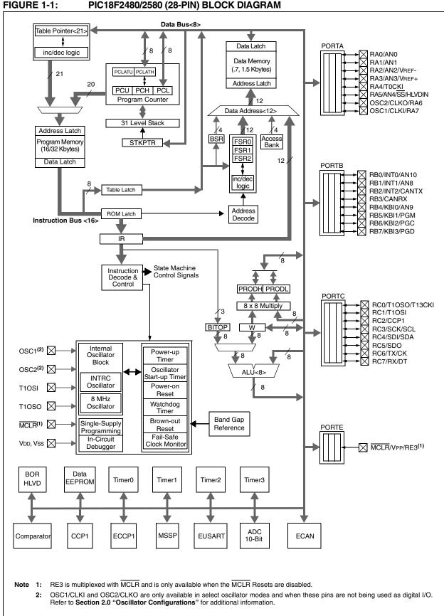
PIC18F2480/2580 (28-PIN) BLOCK DIAGRAM
