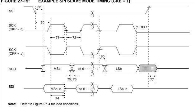
FIGURE 27-15: **EXAMPLE SPI SLAVE MODE TIMING (CKE = 1)**
