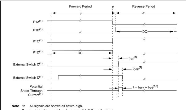
2: t<sub>ON</sub> is the turn-on delay of power switch QC and its driver.
