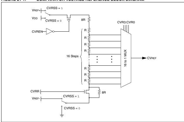
FIGURE 21-1: COMPARATOR VOLTAGE REFERENCE BLOCK DIAGRAM
