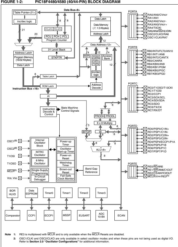
PIC18F4480/4580 (40/44-PIN) BLOCK DIAGRAM FIGURE 1-2:
