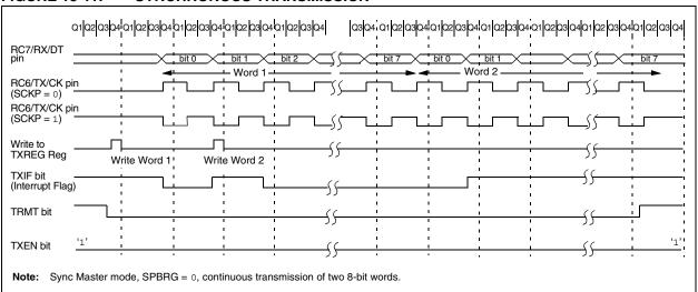
FIGURE 18-12: SYNCHRONOUS TRANSMISSION (THROUGH TXEN)
