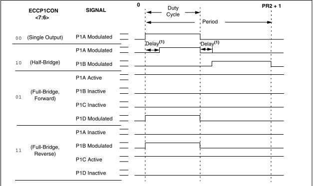
**FIGURE 16-3:** PWM OUTPUT RELATIONSHIPS (ACTIVE-LOW STATE)
