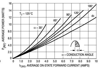
Figure 2. Maximum On-State Power Dissipation
