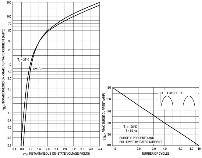
Figure 3. On-State Characteristics
