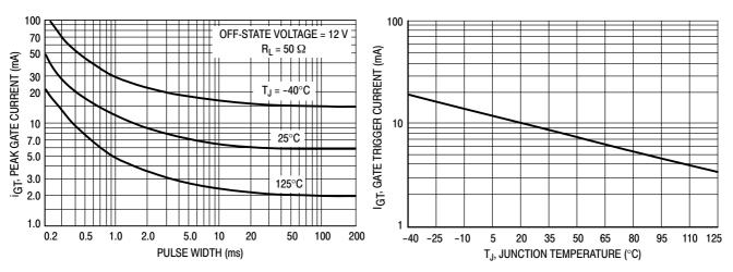
Figure 6. Typical Gate Trigger Current versus Pulse Width
