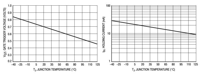
Figure 8. Typical Gate Trigger Voltage versus Junction Temperature
