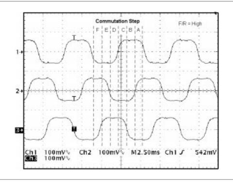
Figure 9. Hall-Effect Commutation Sequence for Counter-Clockwise Rotation
