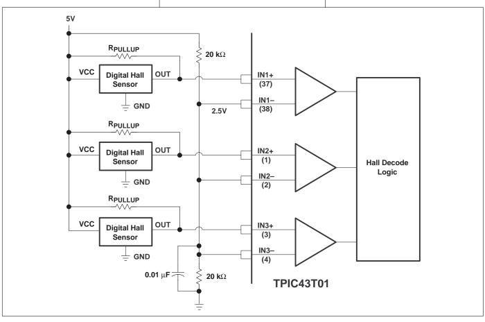
Figure 10. Digital Hall-Effect Sensor Interface
