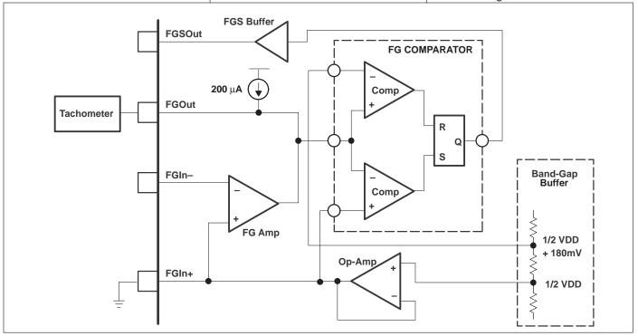
Figure 6. Tachometer Control of FG Interface
