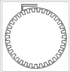
Figure 5. FG Winding Layout Example
