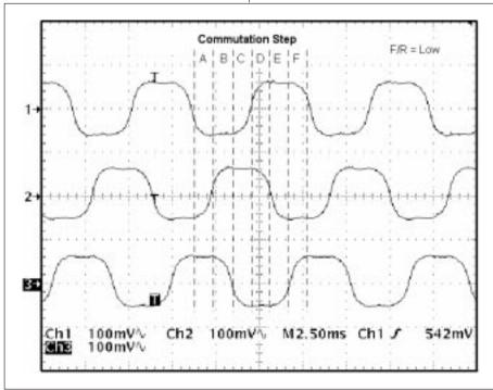
Figure 8. Hall-Effect Commutation Sequence for Clockwise Rotation
