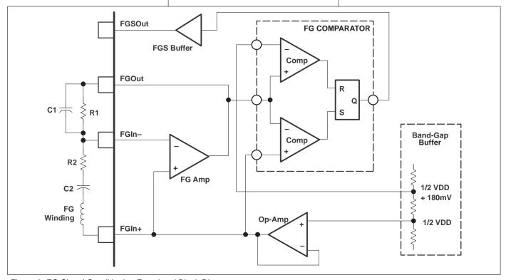
Figure 3. FG Signal Conditioning Functional Block Diagram
