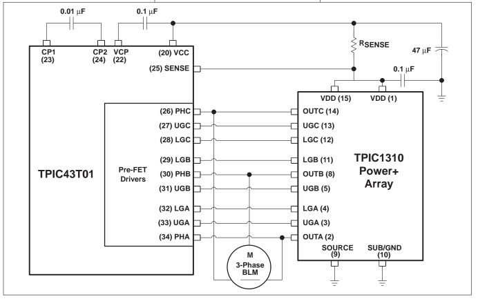
Figure 1. Connections for TPIC43T01 and TPIC1310 Chipset
