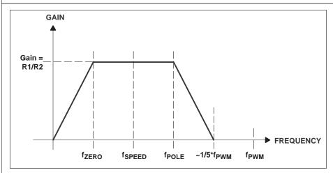
Figure 4. FG Signal Conditioning Input Filter Response
