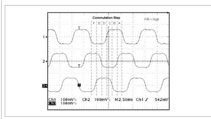
Figure 9. Hall-Effect Commutation Sequence for Counter-Clockwise Rotation
