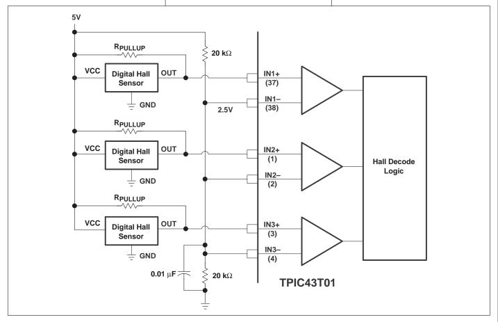
Figure 10. Digital Hall-Effect Sensor Interface
