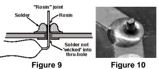
Similarly, a poor joint will result if you do not properly strip and tin the enameled wire leads of inductors *before* the lead is inserted into the PC board for soldering. Enamel coating allowed to remain on the inductor lead can create a joint similar to the rosin joint, preventing the lead from being adequately heated by the soldering iron. Such a joint *cannot* normally be restored by reheating. Remove the lead from the PC board, strip it of all enamel and tin it. Then resolder the joint.
