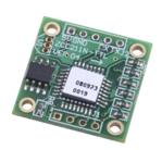
ZCC211N-TTL is a low cost plane electronic compass module. The principle of its work through the reluctance sensors sensing the Earth's magnetic field component, so as to get an azimuth angle. It communicates with PC through TTL. It has high accuracy, stable performance and calibration function. Its Baud rate optional. There are both continuous and inquiry output mode. At the same time it has declination angle and deviation angle compensation function. It can suit different working conditions.
