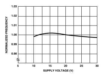
FIGURE 12. FREQUENCY vs SUPPLY VOLTAGE
