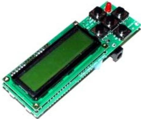
This is the Olimex LPT-MT development board; it has everything the prototype board above includes plus a LCD display and four pushbuttons to experiment with. It costs about \$79.95 plus \$2.95 for the wall-wart power supply.
