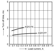
15.-(1) Load current vs. turn off time characteristics
