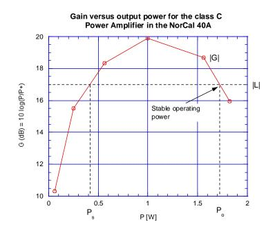
Class C amplifiers will not oscillate if  $P < P_s$ . However, once  $P > P_s$  oscillation may occur if the feedback network meets the phase criterion (11.9).
