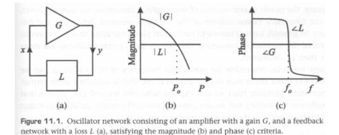
In the NorCal 40A this decreasing |G| occurs because of gain limiting rather than overloading of the amplifier – this scheme yields a cleaner sinusoidal output signal.
