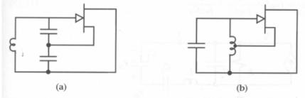
**Figure 11.3.** Colpitts oscillator, with a capacitive-divider feedback network (a), and Hartley oscillator, with inductor feedback (b). The inductor network is usually made by a connection part way down the coil called a *tap*. The amount of feedback is controlled by the position of the tap. In both figures, the bias and load networks are omitted for simplicity.
