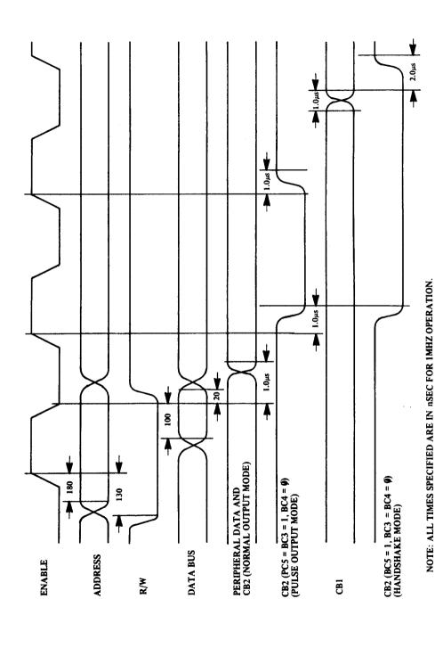
Peripheral B Interface Timing FIGURE 1.27b
