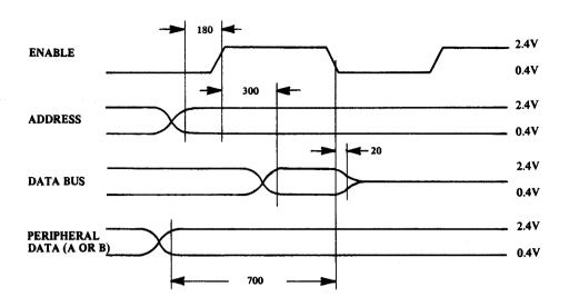
Microprocessor Interface Timing - Read FIGURE 1.26a
