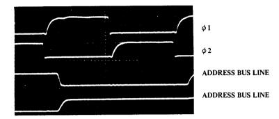
FIGURE 3.7a — Proper Address Lines
