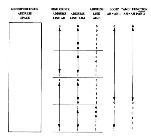
Example of "AND" Function Using High Order Address Lines FIGURE 2.9
