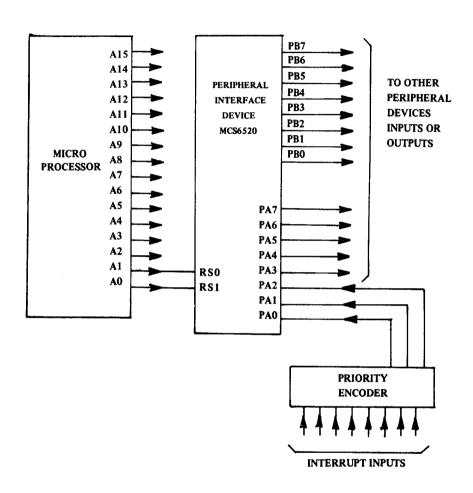
Priority Encoder Connected to Low Order Bits of MCS6520. FIGURE 2.14 a
