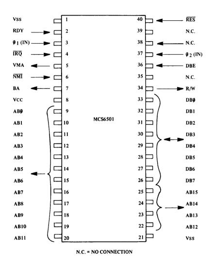
\* VMA IS CONNECTED INTERNALLY TO VCC. THE VMA SIGNAL IS NOT REQUIRED ON THE MCS6501 AS ON THE MC6800, SINCE THE MCS6501 ALWAYS PUTS OUT KNOWN ADDRESSES ON THE ADDRESS BUS.
