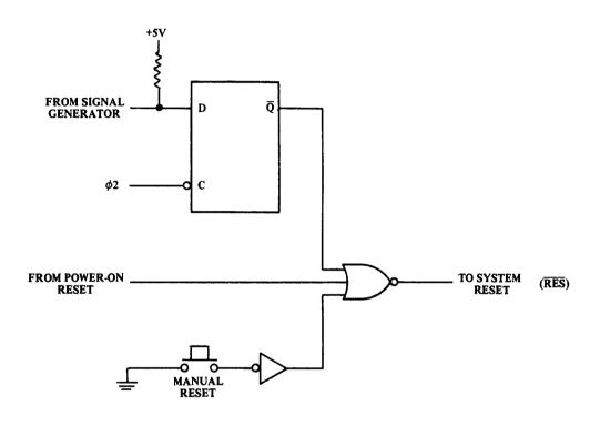
Suggested Configuration For Dynamic Reset Testing. FIGURE 3.5
