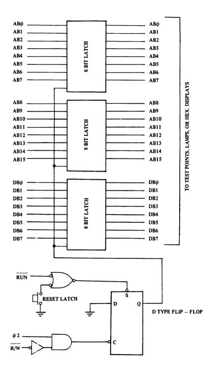
Microprocessor Single Cycle Data Trap FIGURE 3.3
