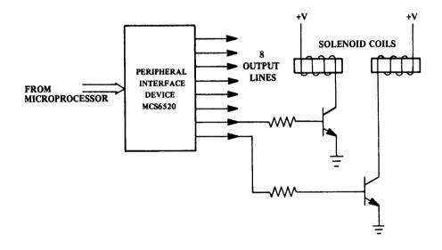
MCS6520 Control of Transistor Driven Solenoids FIGURE 2.2
