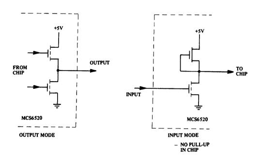
Peripheral I/O Port B Buffer FIGURE 1.28B
