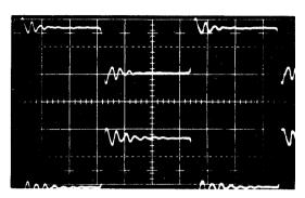
FIGURE 3.6a – Improper Clocks (Note undershoot and overlap)
