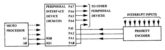
Priority Encoder to Peripheral Interface Scheme FIGURE 2.14 b
