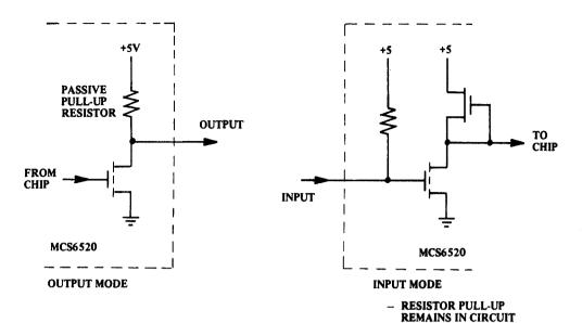
Peripheral I/O Port A Buffer FIGURE 1.28A
