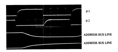
FIGURE 3.7b - Excess Address Line Loading
