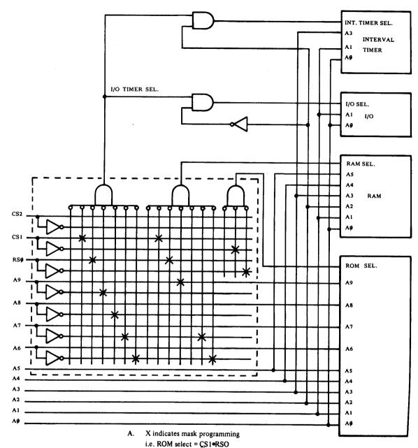
RAM select =  $\overline{CS1} \bullet \overline{RSO} \bullet \overline{A9} \bullet \overline{A7} \bullet \overline{A6}$ I/O TIMER SELECT =  $\overline{CS1} \bullet \overline{RSO} \bullet \overline{A9} \bullet \overline{A9} \bullet \overline{A7} \bullet \overline{A6}$ B. Notice that A8 is a don't care for
