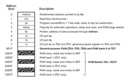
Figure 1. Simplified memory map of PIC's 16C54 through '57.
