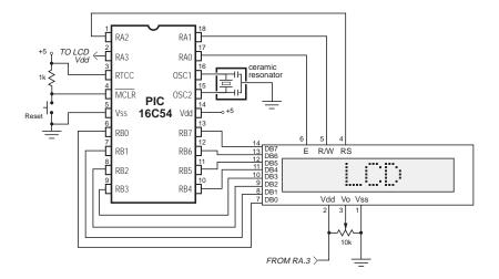
Hitachi LCD modules display the standard ASCII character set, plus selected Japanese, Greek, and math symbols. They operate from a single-ended 5-volt supply, and communicate with a bus or controller through 11 input/output (I/O) lines. The data lines are tri-state; they go into a high-impedance state when the LCD is not enabled.
