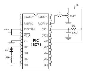
Input Characteristics. The ADC produces a digital output that is proportional to an analog input. A voltage reference determines the input voltage that will produce a full-scale (255) digital output. The voltage reference can be the +5-volt power-supply rail, or some other voltage source between 3 volts and the power supply voltage + 0.3 volts. The ADC is most accurate with a reference voltage of 5.12 volts, according to the manufacturer's specifications.
