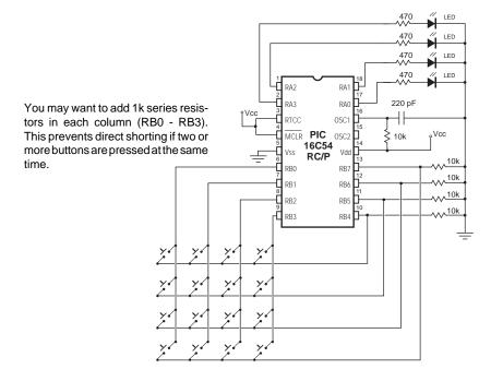
Modifications. In circumstances where electrical noise might be a problem, Microchip's data sheet on the PIC indicates that it might be wise to move the port I/O assignments to the beginning of *scankeys*. The reason is that electrostatic discharge (ESD) from the user's fingertips, or presumably any other strong electrical noise, could corrupt an I/O control register and switch an input pin to output. This would prevent the routine from reading one or more rows of the keypad.
