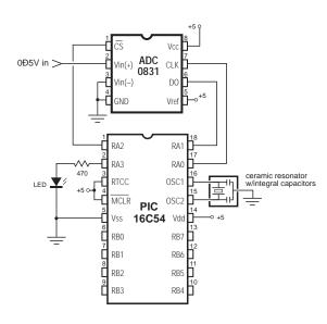
In the example application,  $V_{IN}(-)$  is at ground and  $V_{REF}$  is at +5; however, these values can be as close together as 1 volt without harming accuracy or linearity. You may use diode voltage references or trim pots to set these values.
