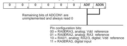
Figure 2. ADC control registers.
