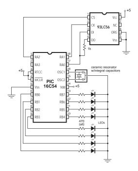
The Microchip 93C56 and 93LC56 electrically erasable PROMs (EEPROMs) are perfect for these applications. They communicate serially via a three- or four-wire bus using a simple synchronous (clocked) communication protocol at rates of up to 2 million bits per
