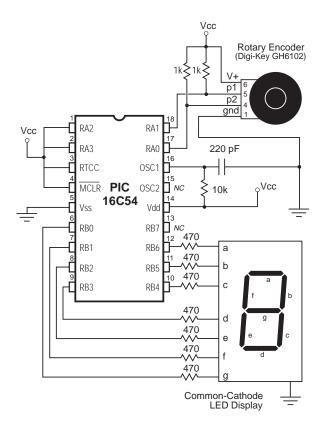
This phase relationship provides the information needed to determine the encoder's direction of rotation (see figure 1).
