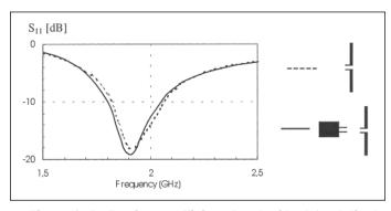
Figure 6. Reflection coefficient for the ideal feed dipole antenna (dotted) and for the dipole feed via the simulated balun (solid).
