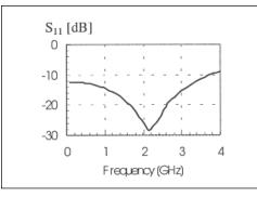
▲ Figure 7. Simulated reflection coefficient s<sub>11</sub>-parameter for the balun where the CPS is terminated by an ideal 80-ohm resistor.
