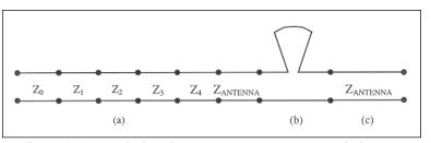
Figure 3. Transmission line model of the balun consisting of the coplanar step impedance waveguide (a), the balun (b), and the coplanar strip line.
