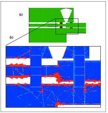
Figure 9. The CPW-to-CPS balun (a). A Close-up picture of the current density where the arrows show the direction and the density of the current at a specific location (b).
