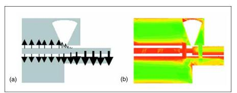
Figure 8. Electrical field pattern for the CPW-to-CPS balun (a). The average current density is shown in (b) where the density at each location is illustrated by IE3D where red indicates the highest and green the lowest current density.
