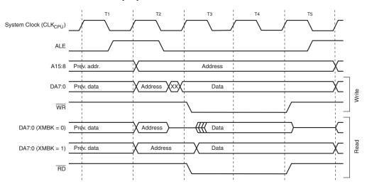
Figure 14. External Data Memory Cycles with SRWn1 = 0 and SRWn0 = 1<sup>(1)</sup>
