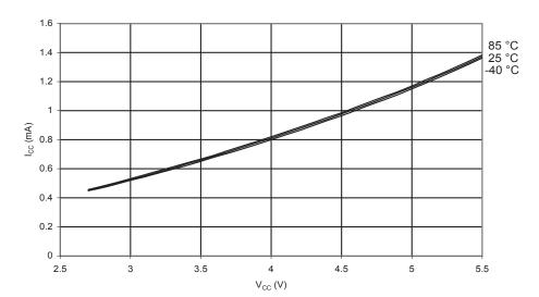
Figure 170. Idle Supply Current vs.  $V_{\text{CC}}$  (Internal RC Oscillator, 1MHz)
