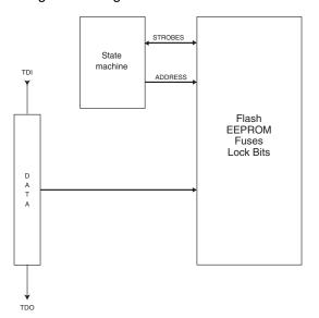
Figure 150. Virtual Flash Page Load Register
