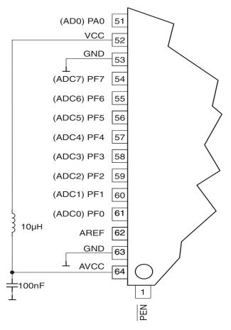
Figure 114. ADC Power Connections
