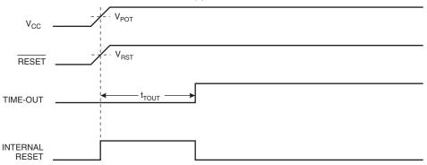
Figure 24. MCU Start-up, RESET Extended Externally
