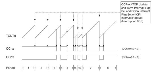
Figure 52. Fast PWM Mode, Timing Diagram
