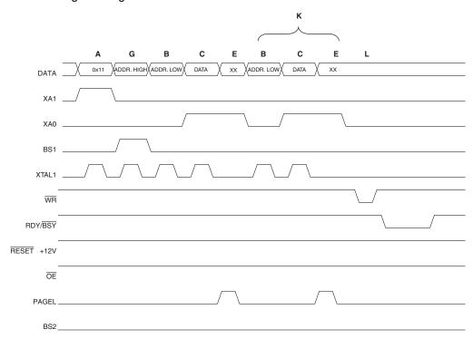
Figure 138. Programming the EEPROM Waveforms
