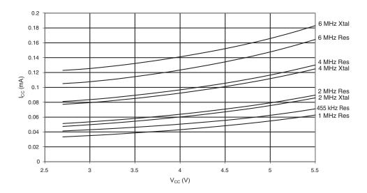
Figure 179. Standby Supply Current vs.  $V_{CC}$  (CKOPT programmed)
