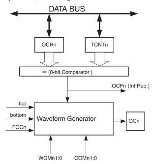
The OCR2 Register is double buffered when using any of the pulse width modulation (PWM) modes. For the normal and Clear Timer on Compare (CTC) modes of operation, the double buff-
