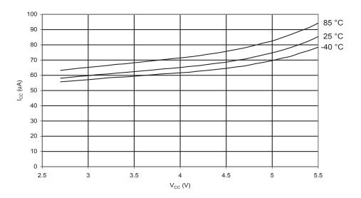
Figure 209. Programming Current vs.  $V_{CC}$
