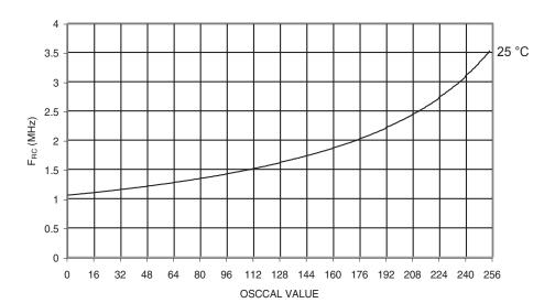
Figure 198. 2MHz RC Oscillator Frequency vs. Osccal Value
