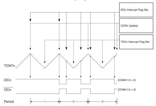
Figure 67. Phase Correct PWM Mode, Timing Diagram
