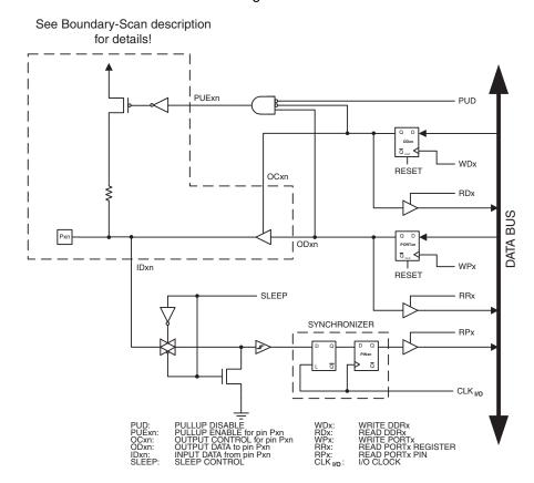
Figure 125. General Port Pin Schematic diagram
