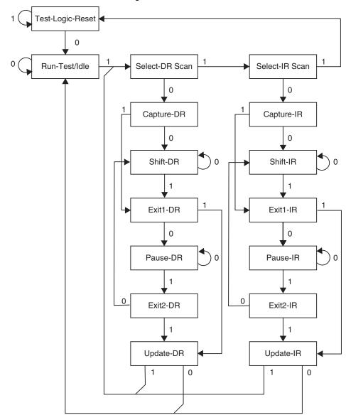
Figure 121. TAP Controller State Diagram
