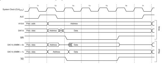
Figure 16. External Data Memory Cycles with SRWn1 = 1 and SRWn0 = 1<sup>(1)</sup>
