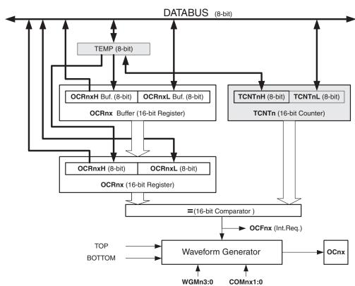
Figure 49. Output Compare Unit, Block Diagram
