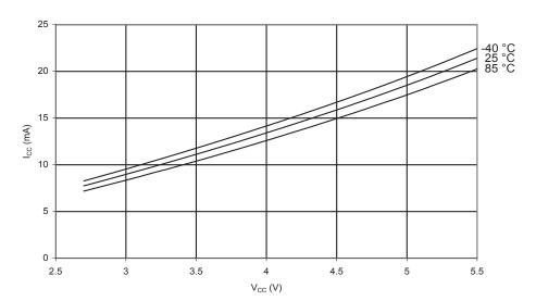
Figure 166. Active Supply Current vs.  $V_{\text{CC}}$  (Internal RC Oscillator, 8MHz)
