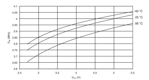
Figure 200. Calibrated 4MHz RC Oscillator Frequency vs.  $V_{\rm CC}$
