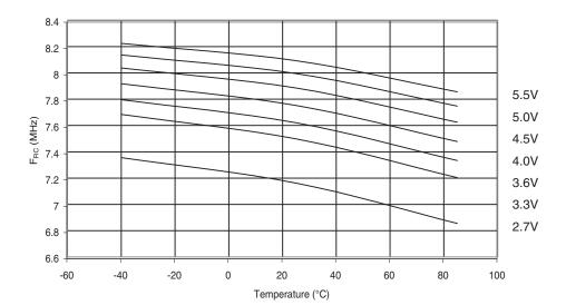
Figure 202. Calibrated 8MHz RC Oscillator Frequency vs. Temperature
