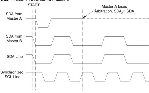
Figure 93. Arbitration Between two Masters
