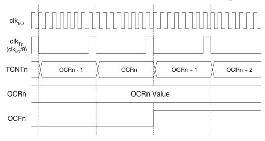
Figure 44 shows the setting of OCF0 and the clearing of TCNT0 in CTC mode.
