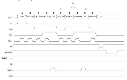
Figure 137. Programming the Flash Waveforms
