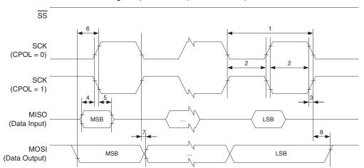
Figure 155. SPI Interface Timing Requirements (Master Mode)
