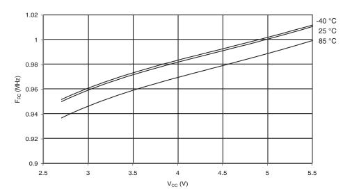
Figure 194. Calibrated 1MHz RC Oscillator Frequency vs.  $V_{\rm CC}$
