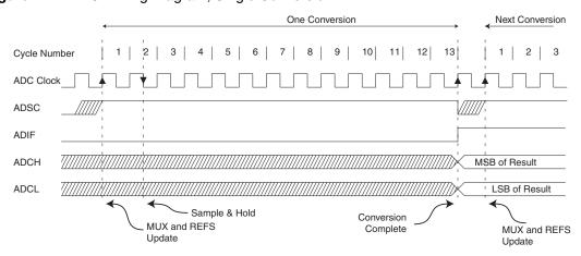
Figure 112. ADC Timing Diagram, Free Running Conversion
