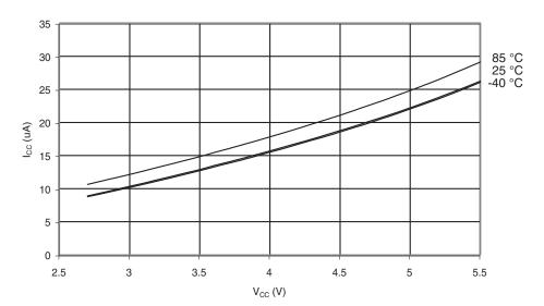
Figure 176. Power-down Supply Current vs.  $V_{\text{CC}}$  (Watchdog Timer Enabled)
