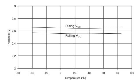
Figure 190. BOD Threshold vs. Temperature (BODLEVEL is 2.7V)
