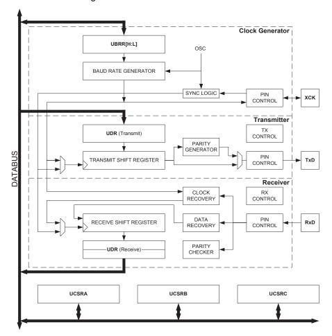
Figure 79. USART Block Diagram
