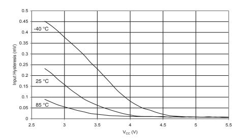
Figure 216. Reset Input Pin Hysteresis vs.  $V_{\rm CC}$
