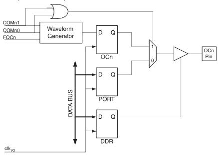
Figure 64. Compare Match Output Unit, Schematic
