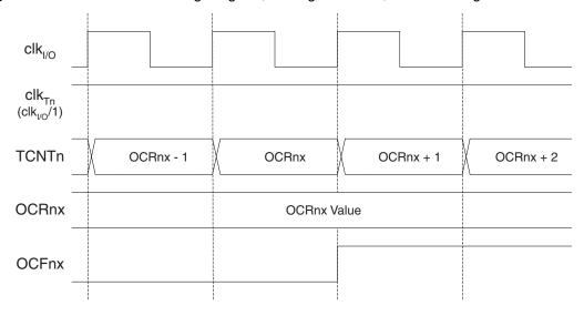
Figure 56 shows the same timing data, but with the prescaler enabled.
