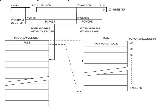
Figure 134. Addressing the Flash During SPM<sup>(1)</sup>
