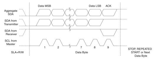
Combining Address and Data Packets Into a Transmission
