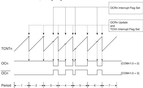
Figure 66. Fast PWM Mode, Timing Diagram
