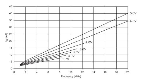
Figure 162. Active Supply Current vs. Frequency (1 - 20MHz)
