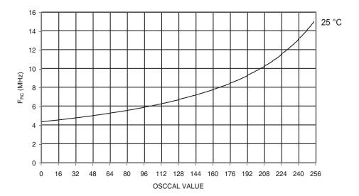
Figure 204. 8MHz RC Oscillator Frequency vs. Osccal Value
