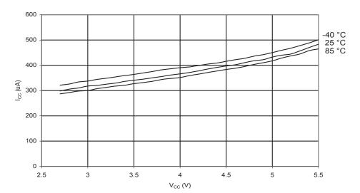
Figure 206. ADC Current vs.  $AV_{CC}$  (ADC at 50kHz)
