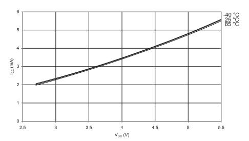
Figure 172. Idle Supply Current vs.  $V_{\text{CC}}$  (Internal RC Oscillator, 4MHz)
