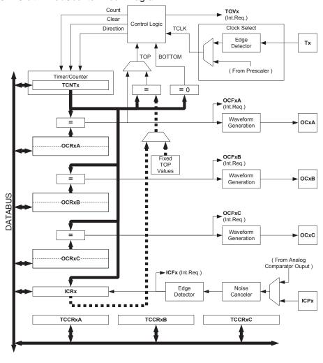
Figure 46. 16-bit Timer/Counter Block Diagram
