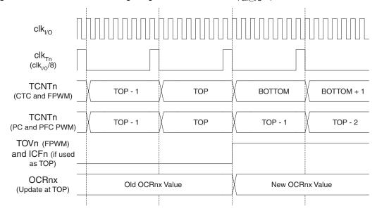
Figure 58. Timer/Counter Timing Diagram, with Prescaler (f<sub>clk I/O</sub>/8)
