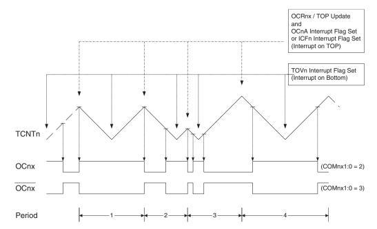
Figure 53. Phase Correct PWM Mode, Timing Diagram
