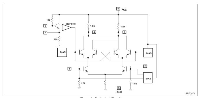
Figure 1. Equivalent Circuit
