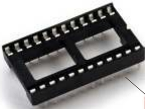
Step 2: BS2 24-pin carrier (note notch position)
