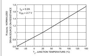
Figure 3. On-Resistance Variation with Temperature.
