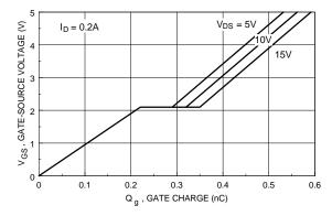
Figure 7. Gate Charge Characteristics.
