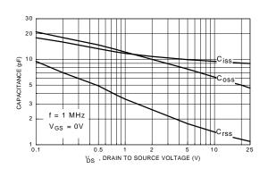
Figure 8. Capacitance Characteristics.
