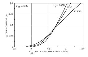
Figure 5. Transfer Characteristics.
