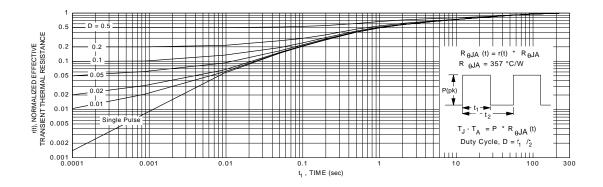
Figure 11. Transient Thermal Response Curve.
