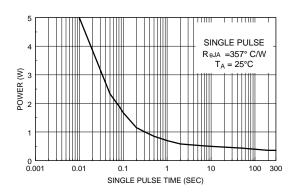
Figure 10. Single Pulse Maximum Power Dissipation.
