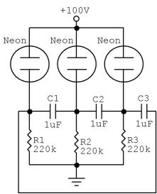
The circuit of the oscillator—as can be seen, there isn't much to it. The basic oscillator block can be extended to as many stages as you wish, but once you exceed three neons, the flash sequence will be pretty much random. gram, there is very little to the circuit. Each neon has its own resistor to limit the current through the lamp, and between each neon/resistor pair is a 1uF, 160 volt bipolar transistor. And that's it!
