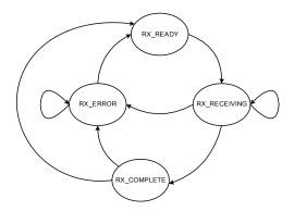
Figure 4: The Receiver State Diagram
