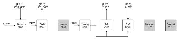
Figure 3: PSoC Digital User Module Placement
