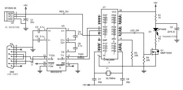
**Figure 2: Codec Schematics**
