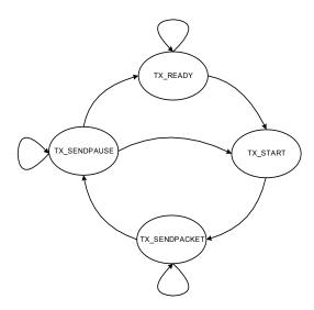
Figure 5: The Transmitter State Diagram
