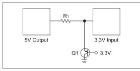
The base-emitter junction of Q1 performs the same function as the diode in a diode clamp circuit. The difference is that only a small percentage of the emitter current flows out of the base of the transistor to the 3.3V rail, the bulk of the current is routed to the collector where it passes harmlessly to ground. The ratio of base current to collector current is dictated by the current gain of the transistor, typically 10-400, depending upon which transistor is used.
