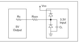
If the clamping diodes are not present, a single external diode can be added to the circuit as shown in Figure 10-2.
