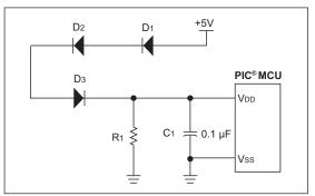
We can also use the forward drop of a series of normal switching diodes to drop the voltage going into the PIC MCU. This can be even more cost-effective than the Zener diode regulator. The current draw from this design is typically less than a circuit using a Zener.
