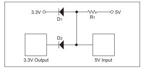
When output voltage specifications are determined, it is done assuming that the output is driving a load between the output and ground for the high output, and a load between 3.3V and the output for the low output. If the load for the high threshold is actually between the output and 3.3V, then the output voltage is actually much higher as the load resistor is the mechanism that is pulling the output up, instead of the output transistor.
