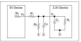
Typically, the source resistance, Rs, is very small (less than  $10\Omega$ ) so its affect on R1 will be negligible provided that R1 is chosen to be much larger than Rs. At the receive end, the load resistance, RL, is very large (greater than 500 k $\Omega$ ) so its affect on R2 will be negligible provided that R2 is chosen to be much less than RL.
