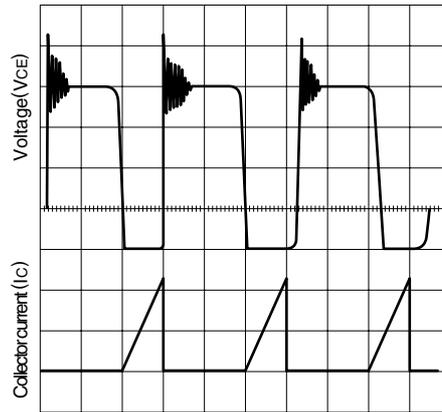
1-transistor forward type converter
