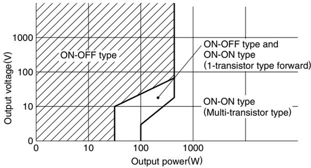
ON-OFF type: For high voltage/small current
