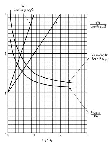
Figure 169. Snubber Energy Loss and the Maximum Overvoltage for the the Optimum Value of Snubber Resistance  $R_S$  and a Function of the Snubber Capacitance  $C_S$  (Courtesy Bill Robbins, University of Minnesota)
