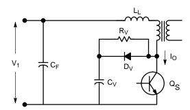
Figure 184. An Overvoltage Snubber
