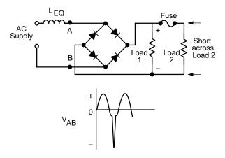
Figure 138. Transients Caused by Load Switching
