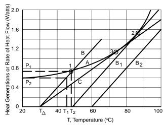
Figure 46. Graphical Analysis of Thermal Runaway
