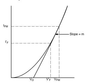
Figure 74. Approximation of a Diode Forward Characteristic for Accurate Calculation of Power Loss when Handling a Sinusoidal Current Waveform
