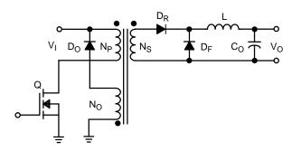
Figure 160. Output Section of a Forward Converter
