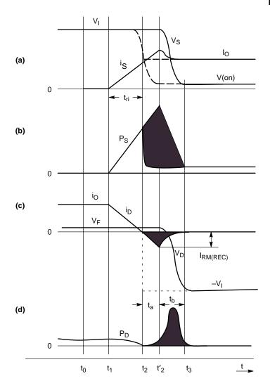
Figure 162. Forced Commutation Waveforms: (a) Power Switch Voltage and Current; (b) Power Switch Dissipation; (c) Diode Voltage and Current; (d) Diode Dissipation.
