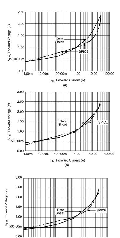
Figure 65. (a) MURH840CT DC Characteristics from Method 1; (b) MURH840CT DC Characteristics from Method 2; (c) MURH840CT DC Characteristics from Method 3
