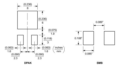
Figure 216. Typical Footprints of Surface-Mount Rectifiers
