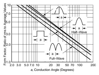
Figure 75. Form Factor for Various Current Waveforms
