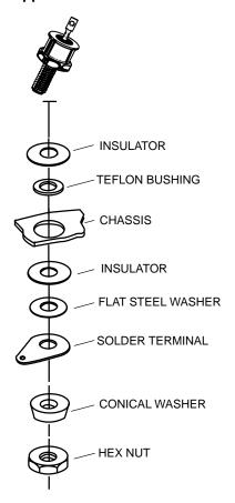
Figure 229. Isolating Hardware Used for a Nonisolated Stud-Mount Package
