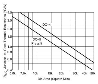
Figure 31. Typical thermal resistance of common rectifier packages having copper material in the heat flow path (data averaged from measurements at ON)
