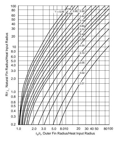
Figure 206. Fin Efficiency  $\eta$  as a Function of  $R/r_i$  and  $r_o/r_i$
