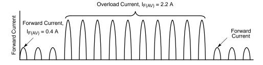
Figure 44. Overload Current Condition Used in Example 2 to Calculate Peak Junction Temperature
