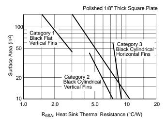
Figure 207. Relation of Surface Area to Thermal Resistance for Categories of Commercial Aluminum Heatsinks as Compared to an Aluminum Plate
