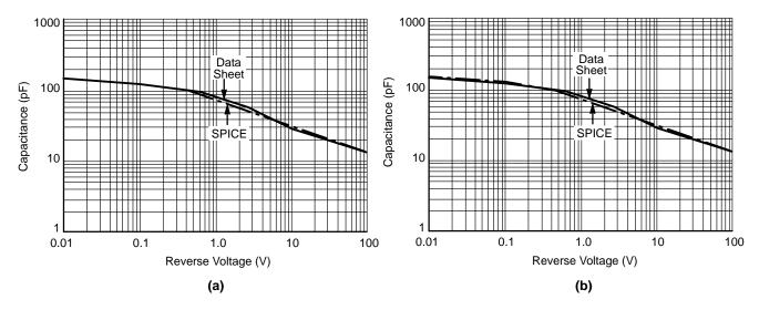
Figure 67. (a) MURH840CT Junction Capacitance Characteristics from Method 1; (b) MURH840CT Junction Capacitance Characteristics from Method 2
