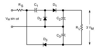
Figure 124. Full-Wave Voltage Tripler Circuit
