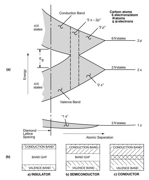
Figure 3. (a) Energy Band Versus Atomic Separation Relationship; (b) Energy Band Gap of Insulators, Semiconductors, and Conductors
