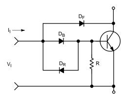
Figure 171. Baker Clamp Configuration
