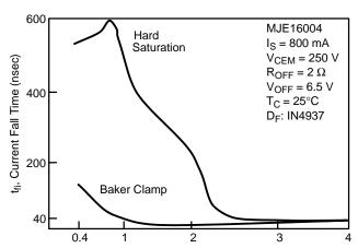
Figure 174. Fall Time with Fixed Drive in a Baker Clamp Circuit
