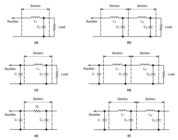
Figure 112. Typical L and π Section Filters: (a) and (b) L–C Filters, Choke Input; (c) and (d) L–C Filters, Capacitor Input; (e) and (f) Filters with Series Resistances
