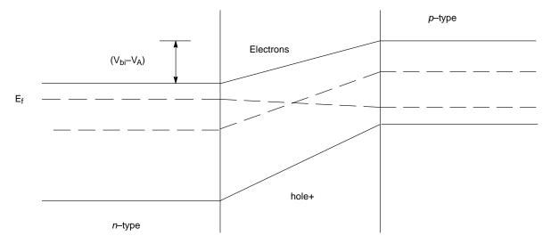
Figure 14. Band Bending Due to Forward Bias Reduces "Built-in" Potential
