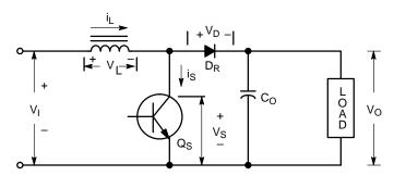
Figure 150. Output Section of a Boost Converter; the Diode Performs Rectification
