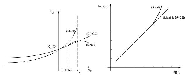
Figure 55. Forward and Reverse-bias Junction C-V Characteristics for the Real, Ideal, and SPICE Diodes
