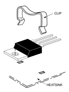
Figure 235. Clip Mounting a TO-220 Mount Package
