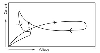
Figure 195. Typical V–I Plot of Semiconductor Material Exhibiting Thermal Breakdown
