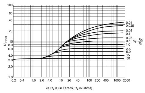
Figure 119. Peak Rectifier Current as a Function of Filter Constants for Full-Wave Voltage Doubler
