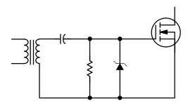
Figure 170. MOSFET Drive Circuit Using dc Restoration to Handle Large Changes in Pulse Duty Cycle
