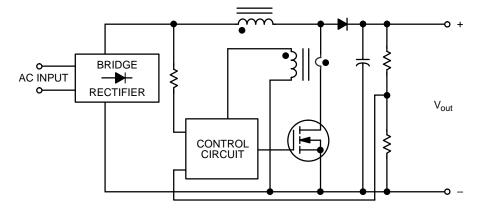
Figure 191. Popular High-Power Factor Rectification Circuit Using a Boost Converter
