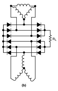
Figure 98. Six-Phase Full-Wave Bridge Circuits
