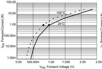
Figure 68. MURH840CT Forward-bias Voltage Temperature Characteristics
