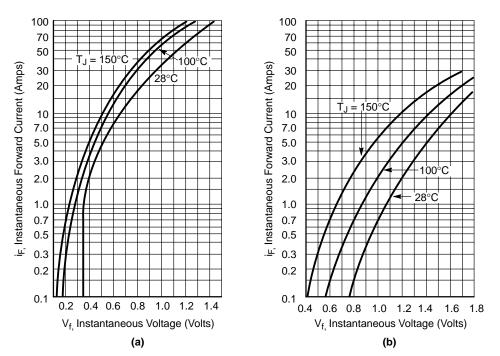
Figure 20. Typical Forward Voltage Characteristic (a) Forward Voltage Characteristic of a 45 Volt Schottky MPR2O4SCT; (b) Forward Voltage Characteristic of 1000 Volt Ultrafast MUR8100E
