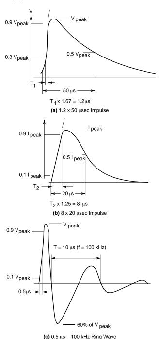
Figure 134. Standard Test Waveforms Defined
