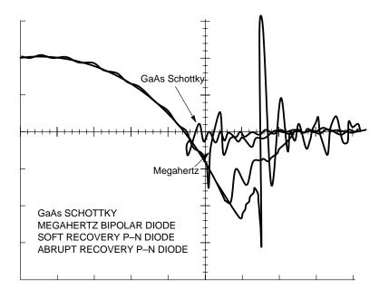
Figure 24. Reverse Recovery Characteristics
