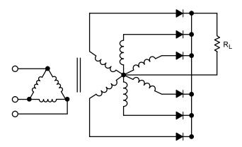
Figure 97. The Six-Phase Star Circuit
