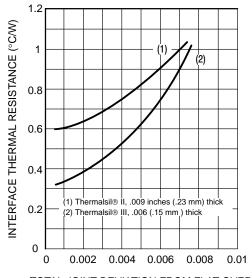
TOTAL JOINT DEVIATION FROM FLAT OVER TO-3 HEADER SURFACE AREA (INCHES)
