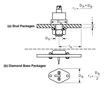
Figure 204. Relation of Semiconductor Device Dimensions to Heat Input Radius r<sub>i</sub>
