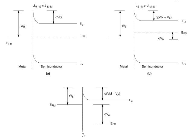
Figure 17. Schottky Barrier Rectifier Energy Band Diagrams (a) No Bias; (b) Forward Bias; (c) Reverse Bias
