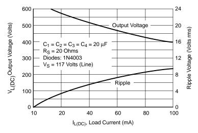
Figure 128. Output Characteristics of a Full-Wave Voltage Quadrupler Circuit.
