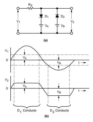
Figure 155. Diode Clipping Circuit and Waveforms when Peak Clipping a Sine Wave:
