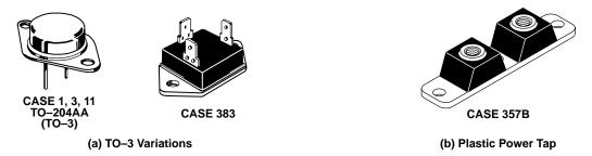
Figure 231. Flange-Mount Packages Used for Rectifiers
