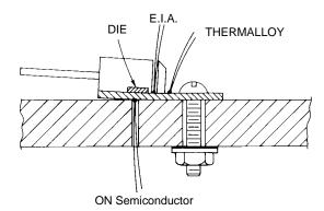
Figure 236. JEDEC TO-220 Package Mounted to Heatsink Showing Various Thermocouple Locations and Lifting Caused by Pressure at One End
