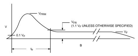
Figure 85. Turn-on Waveform Showing JEDEC Defined Terms.
