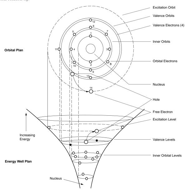
Figure 2. Orbital and Energy Well View of Electrons in Silicon
