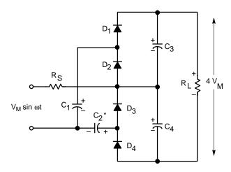
Figure 127. Full–Wave Voltage Quadrupler
