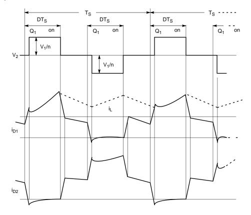
Figure 190. Secondary Waveforms for Push-Pull Converters
