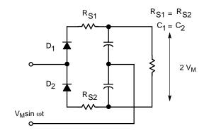
Figure 117. Conventional Full-Wave Doubling Circuit
