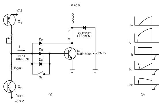
Figure 172. Baker Clamp Circuit for Evaluating High-Voltage Transistors:
