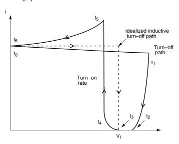
Figure 179. Switching Load Loci for the Buck Converter
