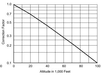
Figure 201. Altitude Correction Factor for Free Convection Heat Transfer
