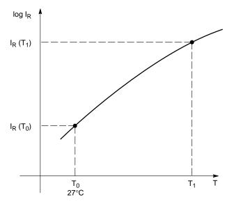
Figure 63. Typical Reverse Leakage Current Temperature Characteristics
