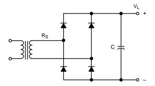
Figure 115. Bridge Circuit Used for Example Design
