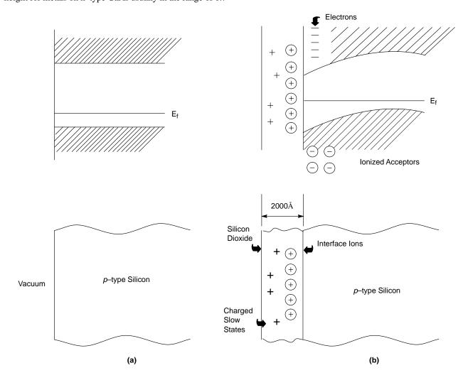
Figure 11. (a) Ideal Surface; (b) Band Rending Due to Energy States in the Forbidden Energy Gap
