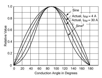
Figure 73. Actual Diode Power Waveforms
