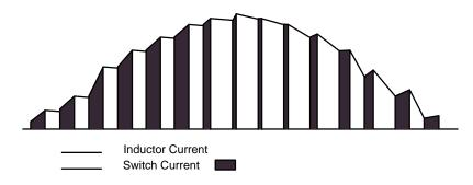
Figure 192. Inductor and Transistor Currents in the Boost Converter Rectifier
