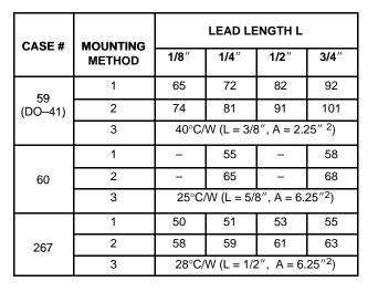
Data shown for the mountings shown is to be used as typical guideline values for preliminary engineering or in case the tie point temperature cannot be measured.
