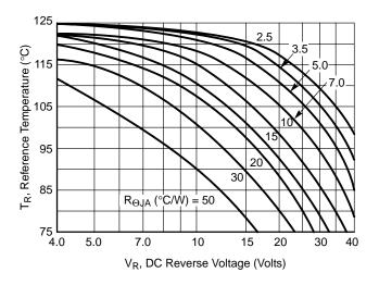
Figure 47. Maximum Reference Temperature for a Schottky Rectifier
