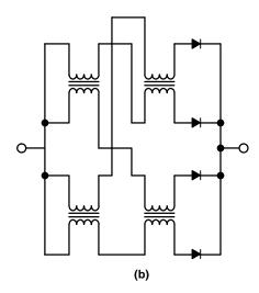
Figure 100. Schemes for Balancing the Current When More than Two Diodes are Required.
