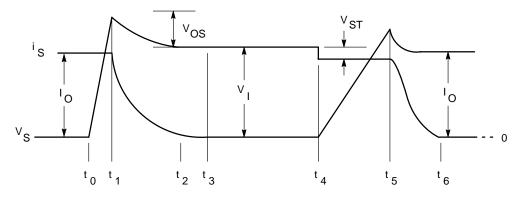
Figure 178. Power Switch Waveforms for the Buck Converter
