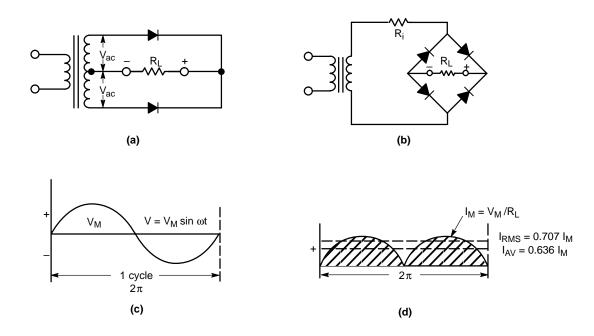
Figure 87. Circuit and Waveshapes for Full-Wave Rectification: (a) Center-Tap Circuit; (b) Bridge Circuit; (c) Input Waveform; (d) Output Waveform
