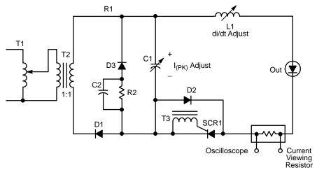
Figure 60. JEDEC Reverse Recovery Time Test Circuit
