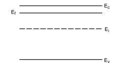
Figure 12. Band Diagram Prior to Junction Formation
