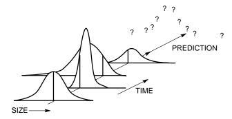
Figure 197. Impact of Assignable Causes on Process Predictability
