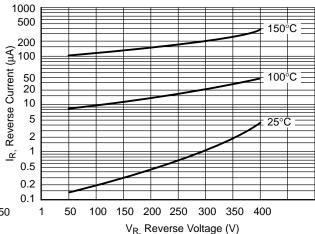
Figure 69. MURH840CT Reverse Leakage Current Temperature Characteristics.
