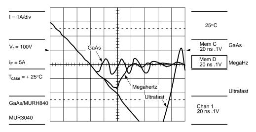
Figure 28. The Reverse Recovery Characteristic of Ultrafast, Megahertz and GaAs at  $T_A = 125$ °C. All Devices Exposed to the Same Test Conditions.
