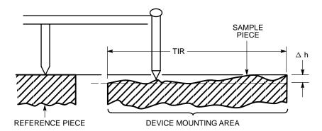
Figure 223. Surface Flatness Measurement
