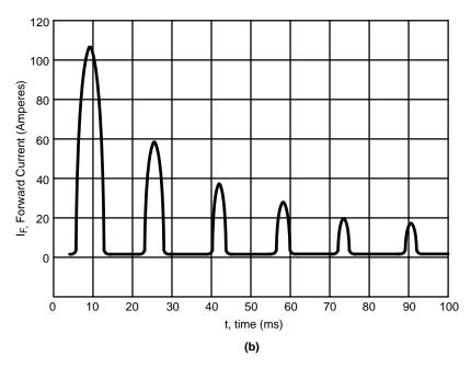
Figure 81. Start up Transients in a Half-Wave Line Operated Rectifier Circuit:
