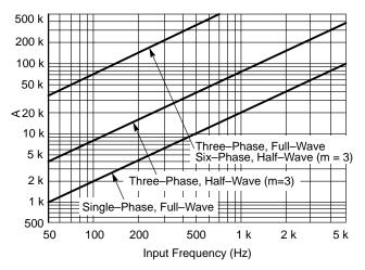
Figure 103. Values for the Constant A Used to Compute Critical Inductance
