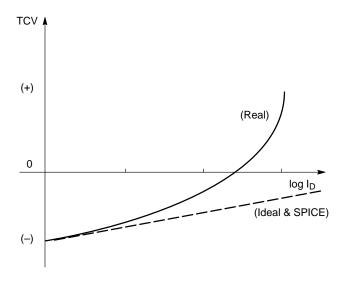
Figure 57. Voltage Temperature Coefficient (TCV)
