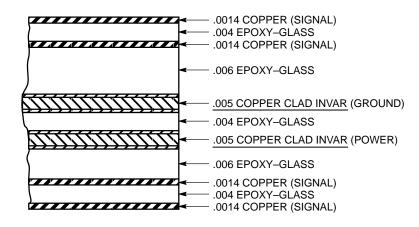
Figure 219. Typical Multilayer Board with Copper-Clad Invar Power and Ground Planes Acting as Constraining Cores
