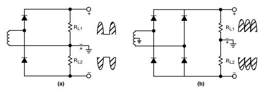
Figure 89. Single-Phase Supplies with Dual Output Voltages: (a) Dual Half-Wave Supply; (b) Dual Full-Wave Supply (a bridge assembly is convenient to use in this application)
