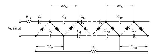
Figure 131. n-Section Voltage Multiplier Circuit
