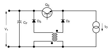
Figure 181. Buck Converter with "Lossless" Turn-on Snubber
