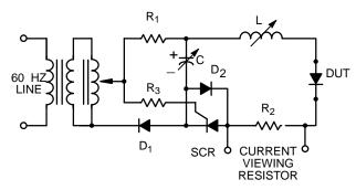
Figure 82. Standard JEDEC Reverse Recovery Test Circuit
