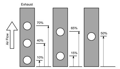
Figure 215. Proper Rectifier Placement for Components having Equal Power Dissipation. Located in this fashion, each semiconductor will operate at the same case temperature and maximize the heatsink performance. In natural convection, mounting must be vertical.
