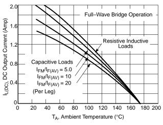
Figure 116. Derating Data for the Example
