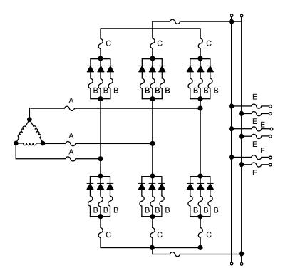
Figure 149. Fuse Placements in a Redundant System
