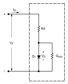
Figure 48. DC Large-signal SPICE Diode Model
