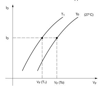
Figure 62. Typical Forward-bias Diode Voltage Temperature Characteristics
