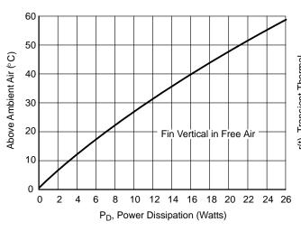
Figure 209. Typical Category 1 Heatsink Natural Correction Thermal Characteristics
