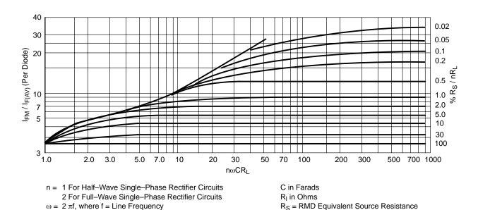
Figure 109. Relation of RMS and Peak to Average Diode Current in Capacitor-Input Circuits (From O.H. Schade, Proc. IRE, Vol. 31, 1943, p. 356)
