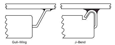
Figure 218. Lead Variations in Surface-mount Components
