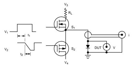
Figure 83. Test Circuit for Ultra-Fast Rectifier Diodes
