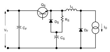
Figure 182. Buck Converter with Dissipative Turn-off Snubber
