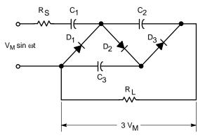
Figure 126. Cascade (Half-Wave) Voltage Tripler
