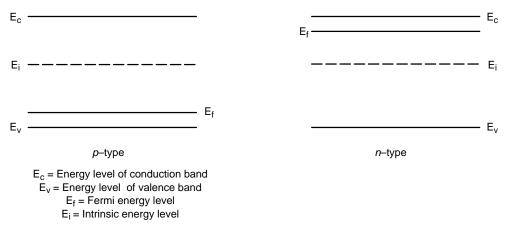
Figure 10. Energy Band Diagram for n-type and p-type with Fermi Levels Shown
