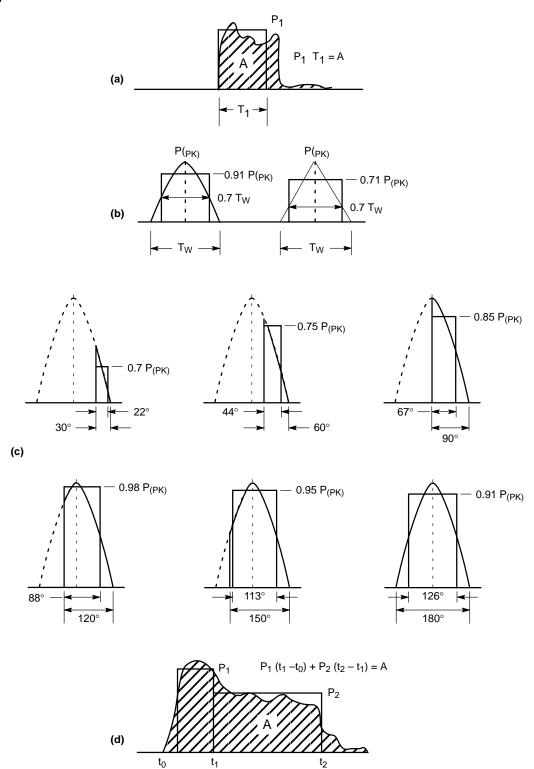
Figure 42. Models for Frequently Encountered Power Pulses (a) Model for Nearly Rectangular Waveform; (b) Models for Sine Wave and Triangular Pulses; (c) Models of SCR Current Waveforms for Various Conduction Angles ( $\propto$ ). Pulses for  $\propto$  >120° are centered with respect to the sine wave. Pulses for  $\propto$  > 90° start at the leading edge; (d) Model for a Complex Waveform
