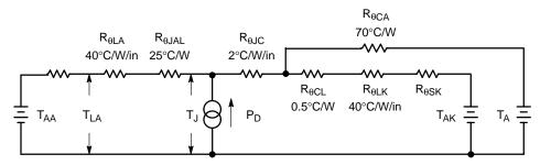
Use of the above model permits calculation of average junction temperature for any mounting situation. Lowest values of thermal resistance will occur when the cathode lead is brought as close as possible to a heat dissipator, as heat conduction through the anode lead is small. Terms in the model are defined as follows:
