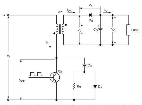
Figure 185. Output Section of a Flyback Converter Having a Transistor Snubber
