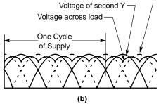
Figure 96. Circuit and Waveforms for the Three-Phase Double Wye Circuit: (a) Circuit; (b) Waveforms
