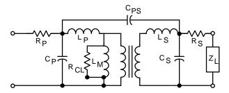
$R_{CL}$  = core loss representation  $L_{m}'$  : primary magnetizing inductance
