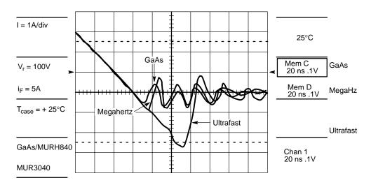
Figure 27. The Reverse Characteristic of Ultrafast, Megahertz and GaAs at  $T_A$  = 25°C. All Devices Exposed to the Same Test Conditions.
