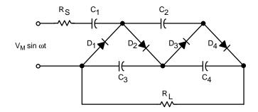
Figure 129. Cascade (Half-Wave) Voltage Quadrupler Circuit
