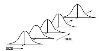
Process "under control" – all assignable causes are removed and future distribution is predictable.
