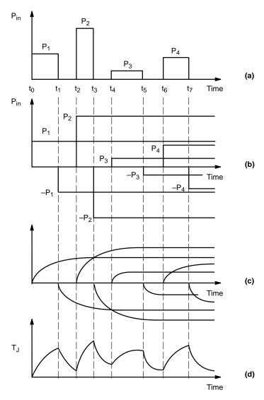
Figure 40. Application of Superposition Principle (a) Input Power; (b) Power Pulses Separated into Components; (c) T<sub>J</sub> Change Caused by Components; (d) Composite T<sub>J</sub>
