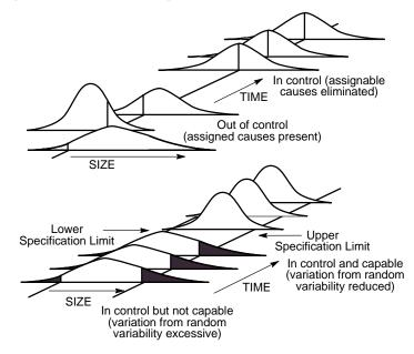
Figure 198. Difference Between Process Control and Process Capability
