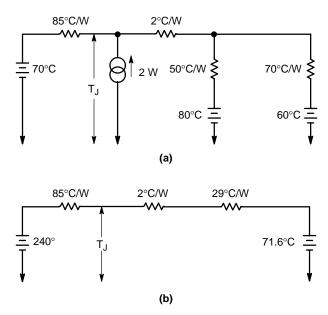
Figure 35. Successive steps in the solution of the example in the text. Thermal problems may be solved by applications of network theorems. (a) Model with example numbers inserted;
