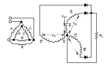
Figure 94. Three-Phase Inter-Star or Zig-Zag Circuit
