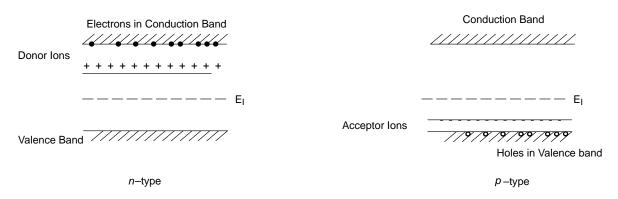
Figure 5. Band Diagram for *n*-type and *p*-type Semiconductors
