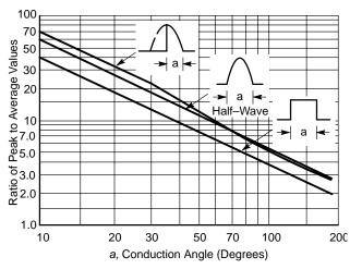
Figure 76. Peak to Average Ratios for Various Current Waveforms
