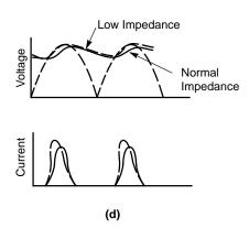
Figure 106. Effects of Circuit Constants and Operating Conditions on Behavior of Rectifier Having a Capacitor–Input Filter: (a) Effect of Load Resistance; (b) Effect of Capacitance; (c) Effect of Transformer Leakage Inductance; (d) Effect of Very Low Diode and Transformer Impedance
