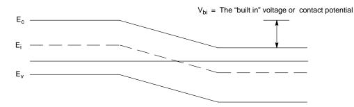
Figure 13. Band Diagram of Ideal Pit Junction
