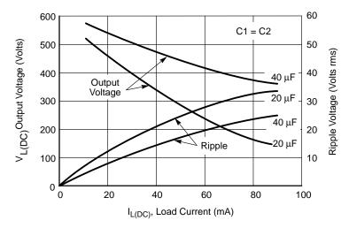
Figure 130. Output Characteristics of the Half-Wave Voltage Quadrupler Circuits
