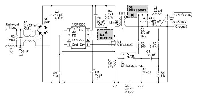
Figure 237. A complete 10 W AC/DC wall adapter featuring an EMI filter.
