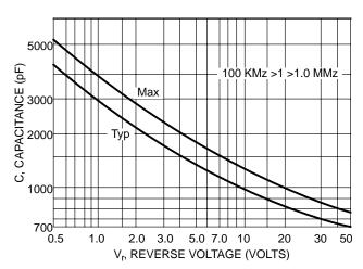
Figure 22. Capacitance Versus Reverse Voltage For Schottky Rectifier
