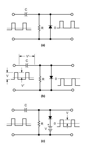
Figure 156. Clamping Circuits and Waveforms; (a) Negative Peaks Clamped to Zero; (b) Positive Peaks Clamped to Zero; (c) Positive Peaks Clamped to V
