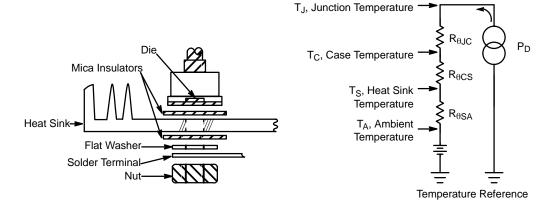
Figure 199. Basic Thermal Resistance Model Showing Thermal to Electrical Analogy for a Semiconductor
