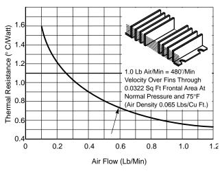
Figure 211. Performance Under Forced Airflow of Typical Category 1 Natural Convection Heatsink
