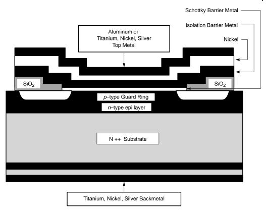
Figure 19. Vertical Structure of Schottky Rectifier
