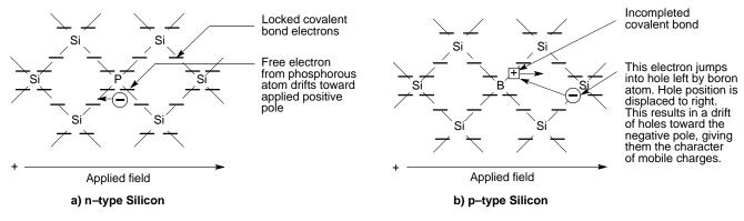
Figure 6. Impurity Atoms in (a) n-type Silicon; (b) p-type Silicon
