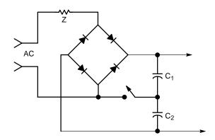
Figure 123. Dual Input Voltage Range Circuit
