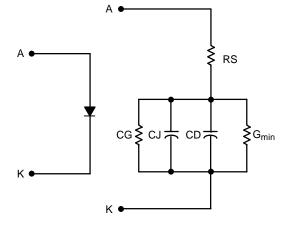
Figure 51. AC Small-signal SPICE Diode Model
