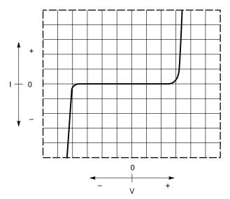
Figure 139. Typical V-I Characteristic of an MOV
