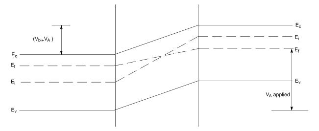
Figure 15. Band Bending Due to Reverse Bias
