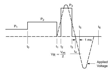
Figure 45. Model of Power Pulses Resulting from the Overload Current Conditions of Figure 44
