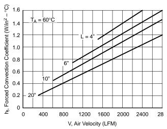
Figure 202. Heat Transfer Coefficient for Forced Air Convection
