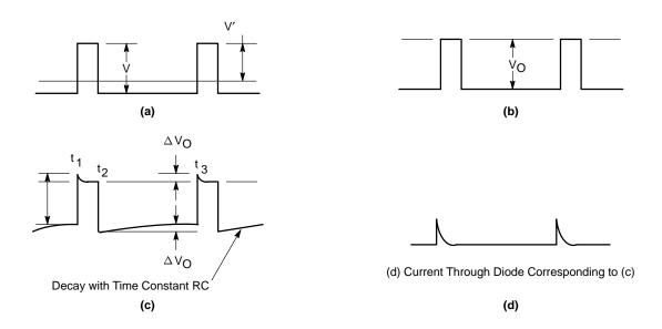
Figure 157. Detailed Waveforms for the Clamping Circuit of Figure 156(b):
