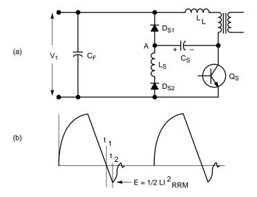
Figure 183. Application of a "Lossless" Snubber of the Resonant Type: (a) circuit; (b) current in D<sub>S2</sub>
