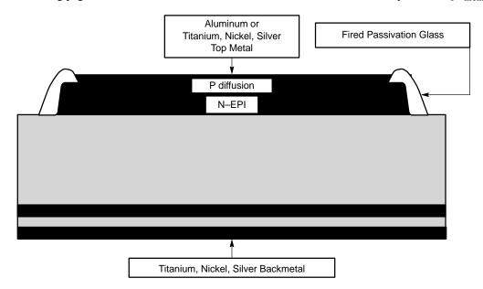
Figure 18. Vertical Structure of pnn+ Rectifier
