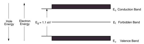
Figure 4. Energy Band Diagram for Intrinsic Silicon
