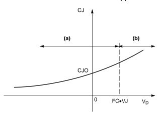
Figure 50. Junction C-V Characteristics of the SPICE **Diode Model**
