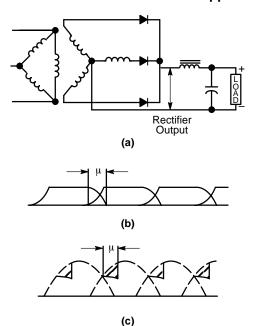
Figure 104. Effect of Transformer Leakage
