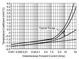
Figure 29.  $\mathcal{O}_{si}$  of Forward Voltage for a Family of Si Diodes
