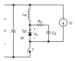
Figure 167. Equivalent Circuit Used to Analyze the Diode Snubber Circuit
