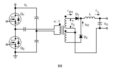
Figure 189. Output Sections of Popular Push–Pull Converters: (a) Center–Tap; (b) Full–Bridge; (c) Half–Bridge
