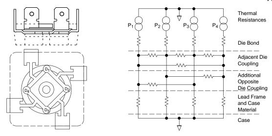
Figure 36. Sketch of Physical Construction and Thermal Model for a Bridge Assembly
