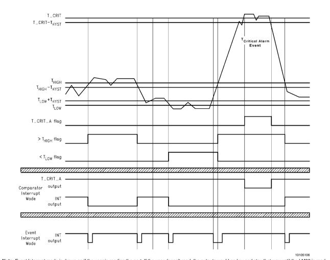
Note: Event Interrupt mode is drawn as if the user is reading the part. If the user doesn't read, the outputs would go low and stay that way until the LM92 is read. Comparator Interrupt Mode is drawn as if the user never reads the part. If the user does read, the outputs will go high once read instruction is executed and, if the fault condition still exists, go low at the end of the next conversion.
