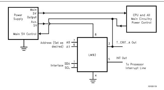
FIGURE 10. ACPI Compatible Terminal Alarm Shutdown. By powering the LM92 from auxiliary output of the power supply, a non-functioning overheated computer can be powered down to preserve as much of the system as possible.
