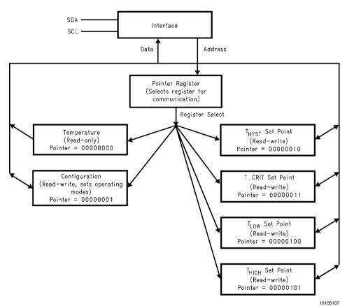
There are four data registers in the LM92, selected by the Pointer register. At power-up the Pointer is set to "00"; the location for the Temperature Register. The Pointer register latches the last location it was set to. In Interrupt Mode, a read from the LM92 resets the INT output. Placing the device in Shutdown mode resets the INT and T\_CRIT\_A outputs. All registers are read and write, except the Temperature register which is read only.
