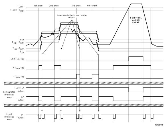
Note: Event Interrupt mode is drawn as if the user is reading the part. If the user doesn't read, the outputs would go low and stay that way until the LM92 is read.
