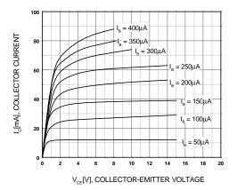
Figure 1. Static Characteristic
