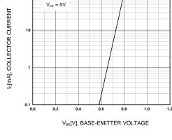
Figure 2. Transfer Characteristic
