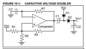
**Note:** The output voltage of a capacitive double is unregulated and will sag with increasing load current. Typically, the output is modeled as a voltage source with a series resistance (see Figure 10-2).
