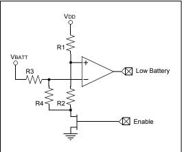
The comparator will trip when the battery voltage, VBATT = 5.7V: R1 = 33k, R2 = 10k, R3 = 39k, R4 = 10k, VDD = 5V.
