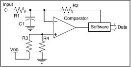
In operation, the feedback output from the software is a time sampled copy of the comparator output. In normal operation, the modulator output generates a PWM signal which is inversely proportional to the input voltage. As the input voltage increases, the PWM signal will drop in duty cycle to compensate. As the input decreases, the duty cycle rises.
