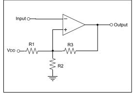
To calculate the resistor values required, first determine the high and low threshold values which will prevent chatter (VTH and VTL). Using VTH and VTL, the average threshold voltage can be calculated using the equation.
