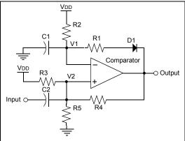
To design the one-shot, first create the hysteresis feedback using the techniques from TIP #3. Remember to set the low threshold below 0.7V. Next, choose values for R2 and C1 using Equation 7-1.
