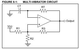
To design a multi-vibrator, first design the hysteresis feedback path using the procedure in TIP #3. Be careful to choose threshold voltages (VTH and VTL) that are evenly spaced within the common mode range of the comparator and centered on VDD/2. Then use VTH and VTL to calculate values for RT and CT that will result in the desired oscillation frequency Fosc. Equation 8-1 defines the relationship between RT, CT, VTH, VTL and Fosc.
