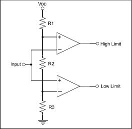
Resistors R1, R2 and R3 form a voltage divider which generates the high and low threshold voltages. The outputs HIGH LIMIT and LOW LIMIT are both active high, generating a logic one on the HIGH LIMIT output when the input voltage rises above the high threshold, and a logic one on the LOW LIMIT output when the input voltage falls below the low threshold.
