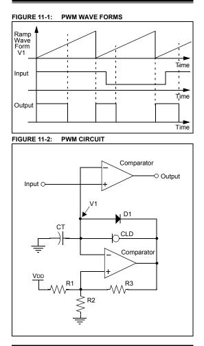
To design a PWM generator, start with the design of a ramp wave multi-vibrator using the design procedure from TIP #9. Choose high and low threshold voltages for the multi-vibrators hysteresis feedback that are slightly above and below the desired PWM control voltages.
