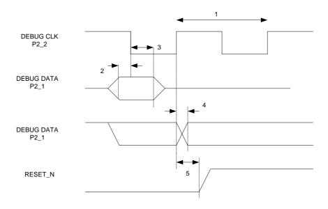
Figure 2: Debug Interface AC Characteristics
