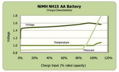
(Fig. 12) Increasing Battery Pressure
