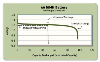
(Fig. 6) Typical Discharge Profile / NiMH Battery
