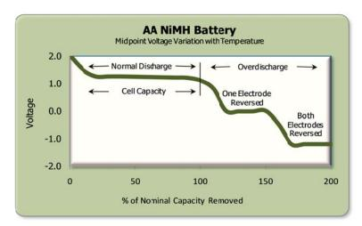
(Fig. 11) Nickel-Metal Hydride Battery Polarity Reversal Voltage Profile
