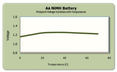
(Fig. 7) Midpoint Voltage Variation with Temperature
