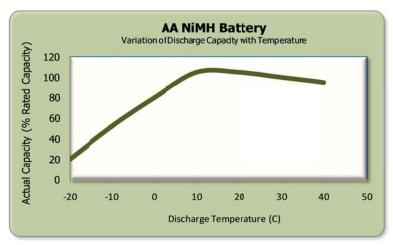
(Fig. 9) Variation of Discharge Capacity with Temperature
