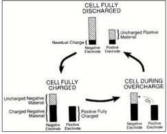
(Fig. 3) Relative Electrode Balances During Discharge/Charge/Overcharge
