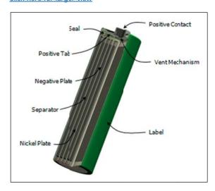
(Fig. 1) Typical NiMH Battery
