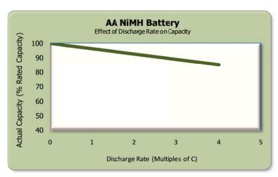
(Fig. 10) Effect of Discharge Rate on Capacity
