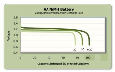
(Fig. 8) Voltage Profile Variation with Discharge Rate
