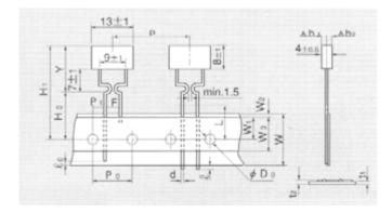
taped version for MPC76 / MPC70 (2W)
