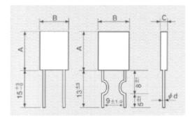
a) left straight leads standard version MPC76 / MPC70 (2W) + MPC75 / MPC71 (5W)
