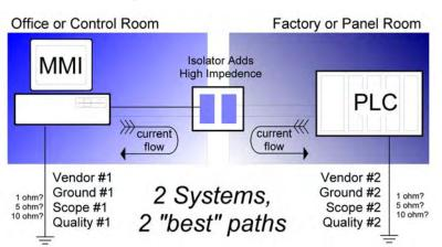
own ground is your own problem. *Galvanic isolation breaks the ground path by using air-gaps, transformers, and/or optical devices. Galvanic isolation allows data to flow between systems, but not electrical current.* This protects your equipment, your warranty repair budget, and your reputation.
