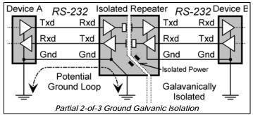
path. 2-port isolation does present another problem; if the isolated repeater shares a DC power supply with other devices, then faults creating surges in the common power supply could effect device A through the isolated repeater.
