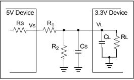
Typically, the source resistance, Rs, is very small (less than 10 ohms) so its affect on  $R_1$  will be negligible provided that  $R_1$  is chosen to be much larger than Rs. At the receive end, the load resistance, RL, is very large (greater than 500 k ohms) so its affect on  $R_2$  will be negligible provided that  $R_2$  is chosen to be much less than RL.
