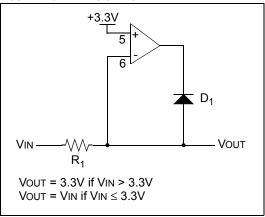
Because the clamping is performed by the op amp, there is no affect on the power supply. The impedance presented to the low voltage circuit is not improved by the op amp, it remains  $R_1$  in addition to the source circuit impedance.
