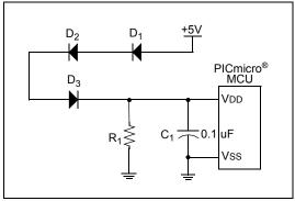
We can also use the forward drop of a series of normal switching diodes to drop the voltage going into the PICmicro MCU. This can be even more cost-effective than the Zener diode regulator. The current draw from this design is typically less than a circuit using a Zener.
