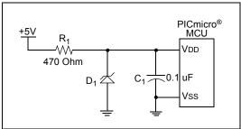
A simple, low-cost 3.3V regulator can be made out of a Zener diode and a resistor as shown in Figure 2-1. In many applications, this circuit can be a cost-effective alternative to using a LDO regulator. However, this regulator is more load sensitive than a LDO regulator. Additionally, it is less energy efficient, as power is always being dissipated in  $R_1$  and  $D_1$ .
