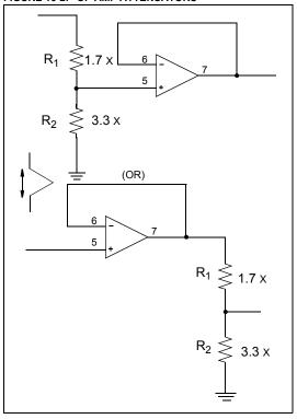
If the resistor divider is before the unity gain follower, then the lowest possible impedance is provided for the 3.3V circuits. Also, the op amp can be powered from 3.3V, saving some power. If the X is made very large, then power consumed by the 5V side can be minimized.
