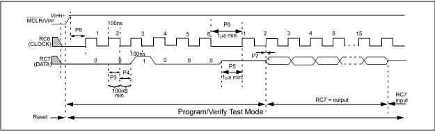
FIGURE 5-3: INCREMENT ADDRESS COMMAND (PROGRAM/VERIFY)
