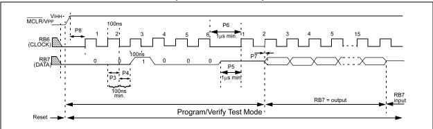
FIGURE 5-3: INCREMENT ADDRESS COMMAND (PROGRAM/VERIFY)
