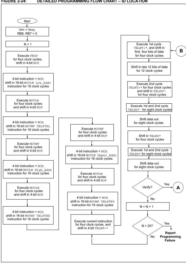
**FIGURE 2-24: DETAILED PROGRAMMING FLOW CHART - ID LOCATION**
