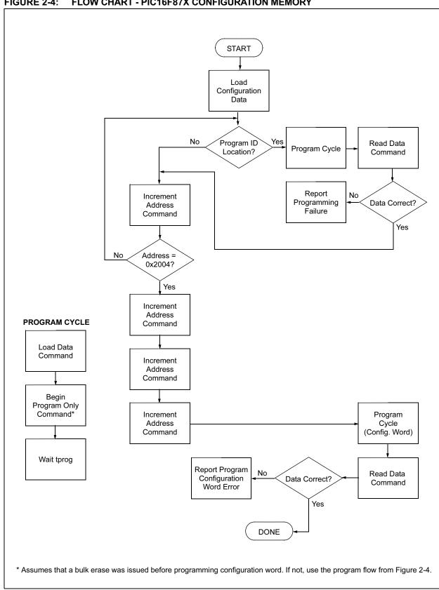
FIGURE 2-4: FLOW CHART - PIC16F87X CONFIGURATION MEMORY
