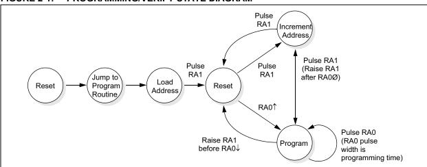
FIGURE 2-1: PROGRAMMING/VERIFY STATE DIAGRAM
