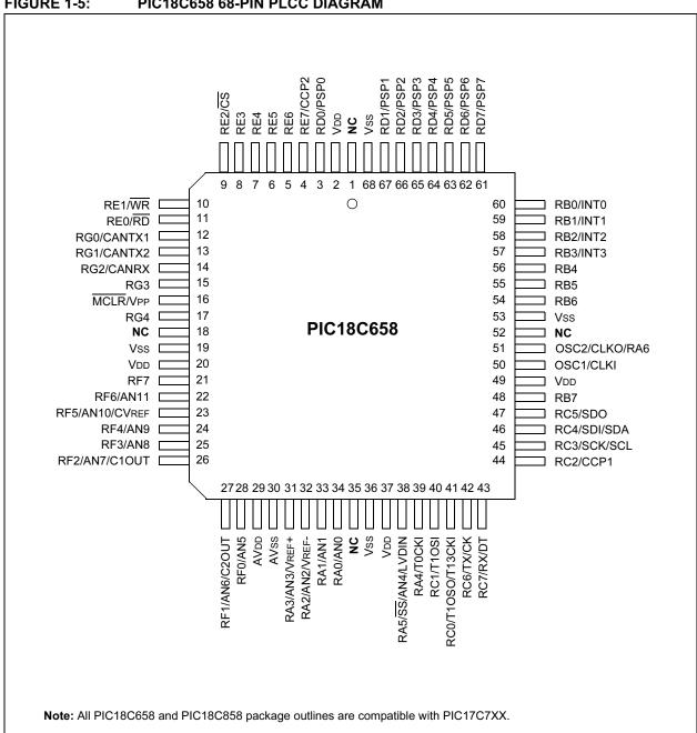
FIGURE 1-5: PIC18C658 68-PIN PLCC DIAGRAM
