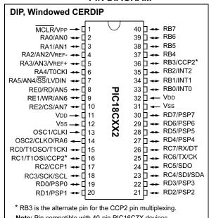
Note: Pin compatible with 40-pin PIC16C7X devices.
