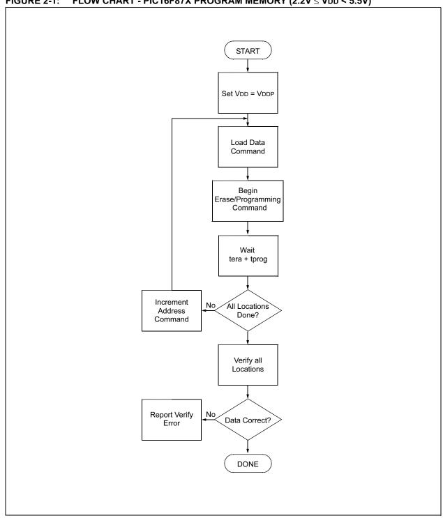
FIGURE 2-1: FLOW CHART - PIC16F87X PROGRAM MEMORY (2.2V ≤ VDD < 5.5V)
